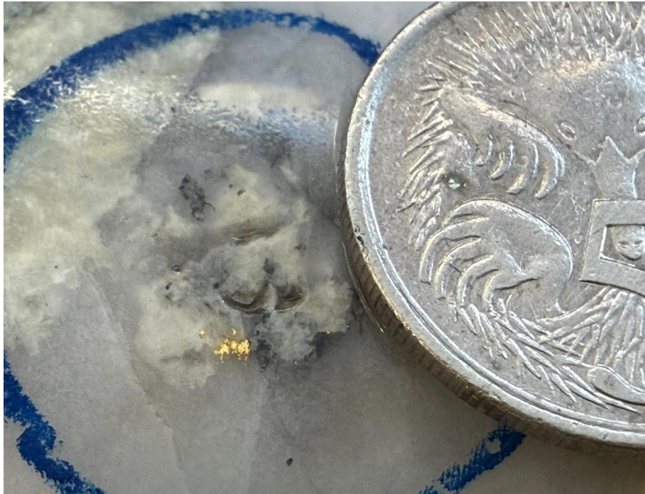
Figure 5 Trace of visible gold in BMDD008 at 246.3m in the Morning Glory Zone
