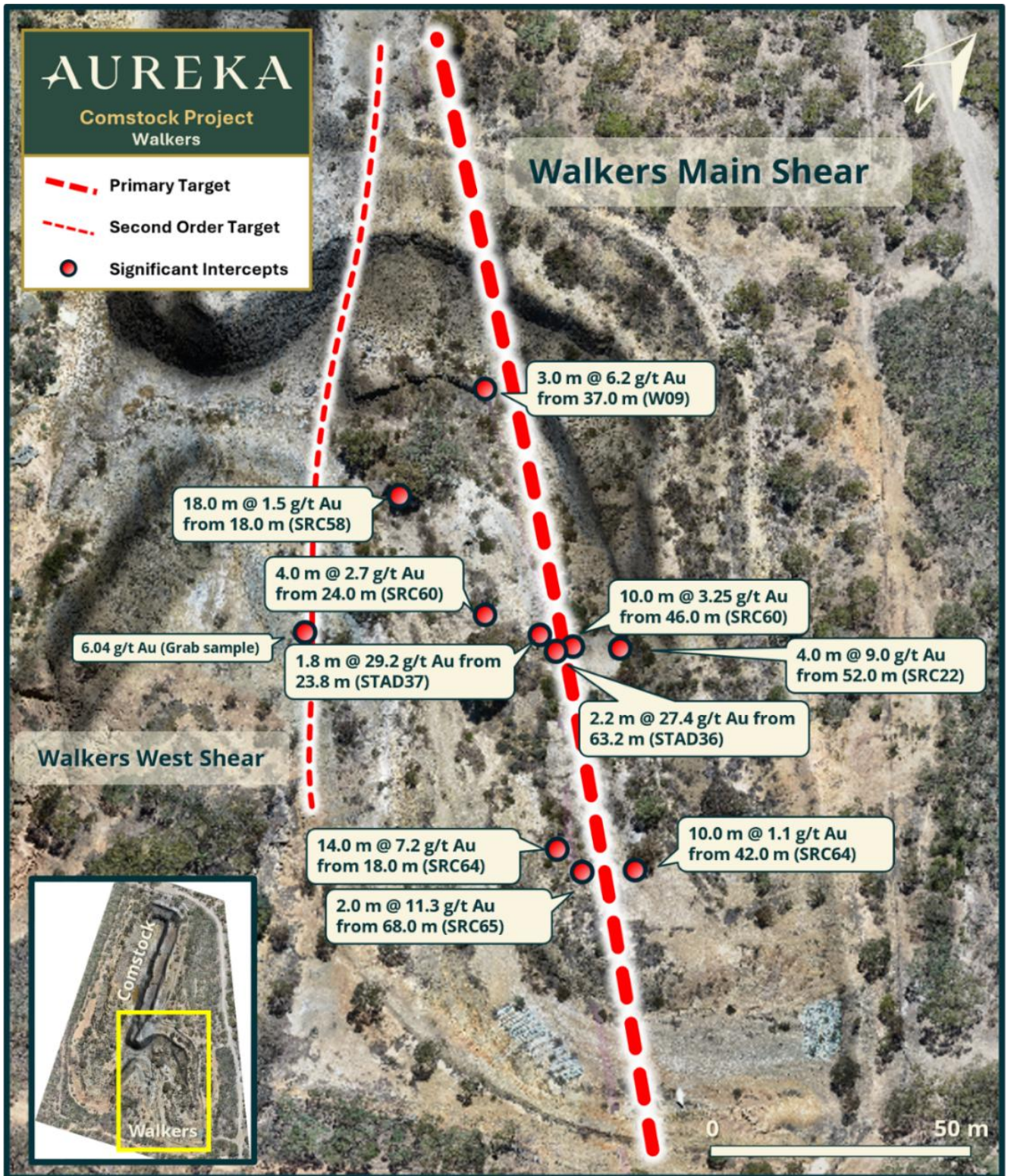
Figure 3 – Plan View of the Walkers sub-pit and the Walkers main Shear with legacy drill intercepts projected to pit floor surface 12 . Historical legacy drilling has been re-published with JORC Tables in this release refer Appendix A and B.
