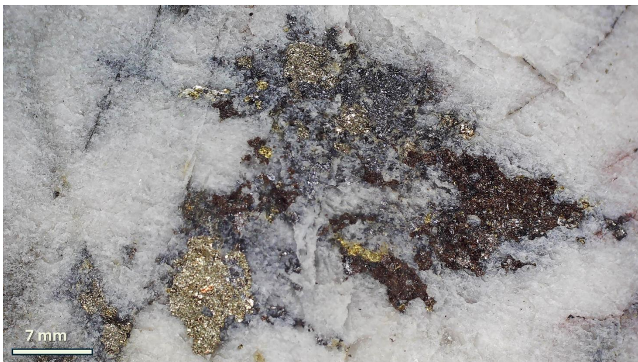
Figure 1: Microscope image of quartz hosted Galena-Sphalerite-Chalcopyrite-Pyrite aggregates hosting Au and Ag mineralisation (0.3m @ 1.91g/t Au and 650g/t Ag from 192m) 5 .
