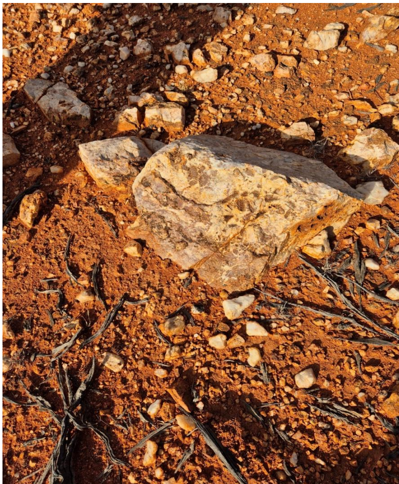
Figure 3 – Brecciated quartz with sulphides cast in proximity of Ballard Fault
