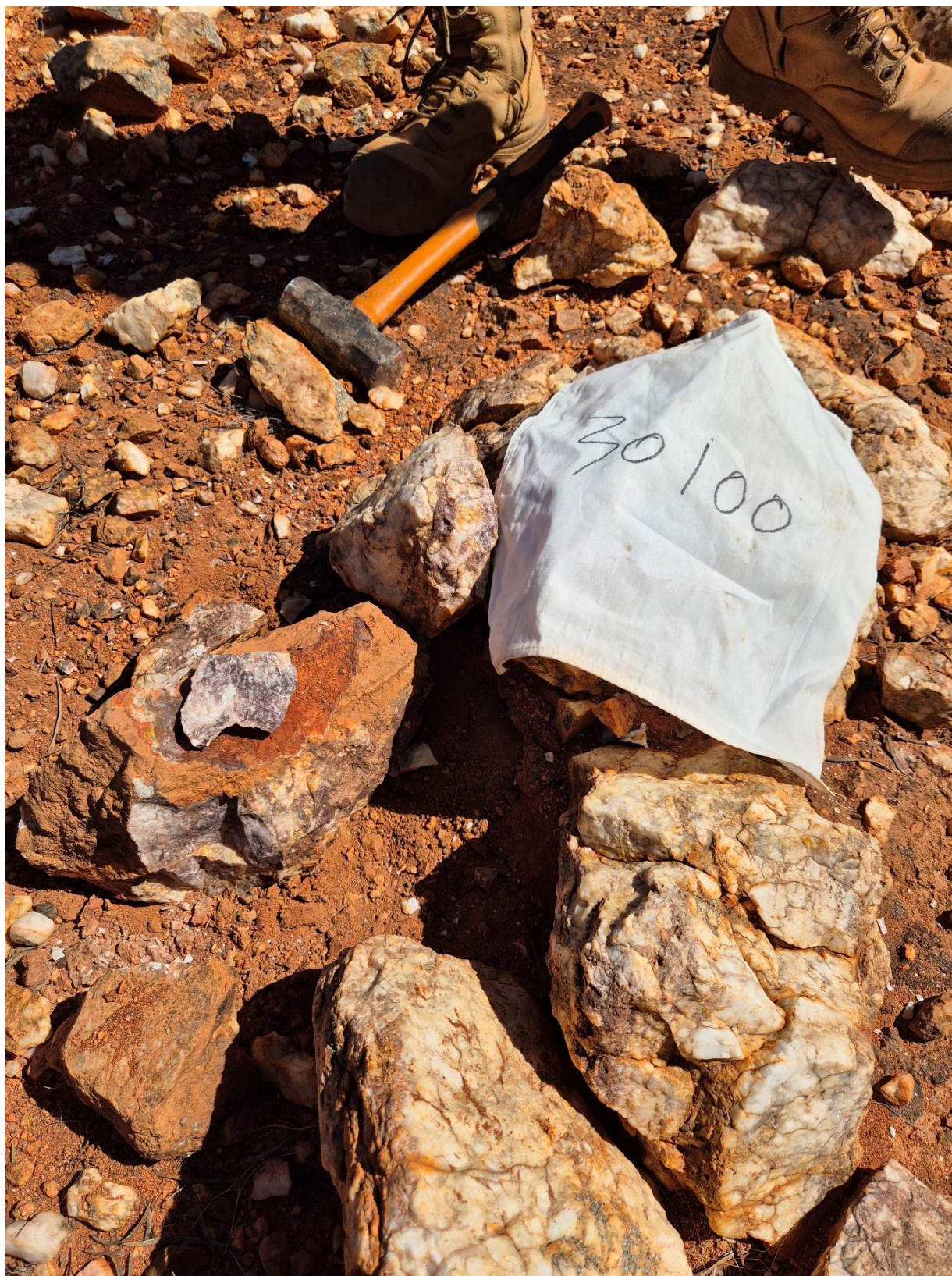
Figure 4 – Ferruginous quartz veins in the Waroonga Shear
