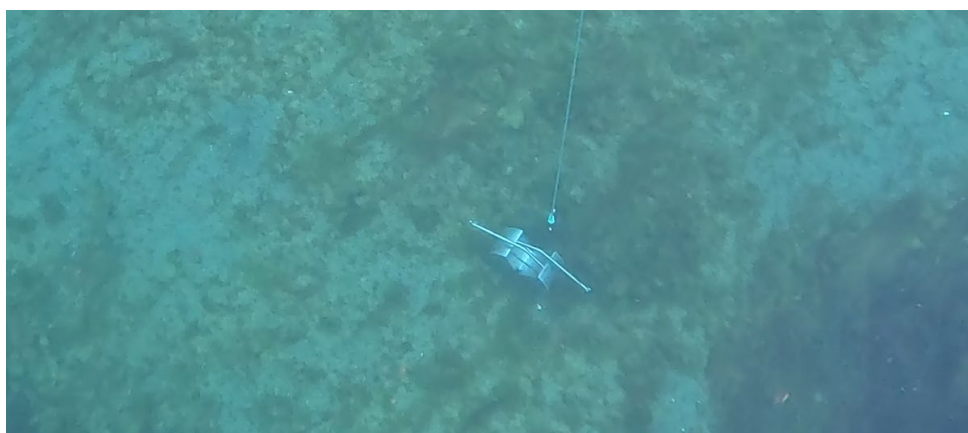
Figure 20. Photograph of the Van Veen grab sampler collecting an unconsolidated sediment sample from the nearshore ocean floor during the 2026 exploration program.
