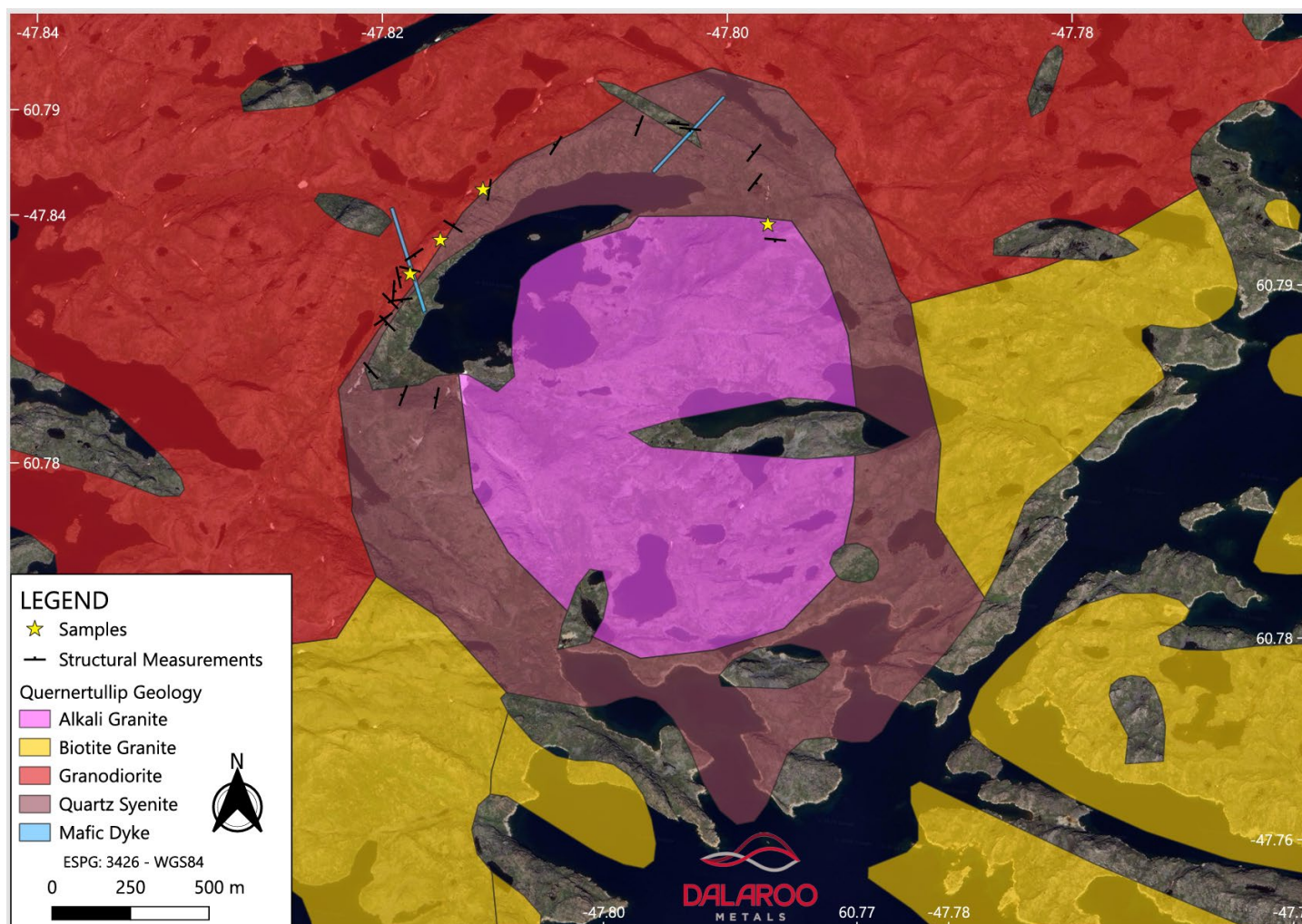
Figure 8. Geological mapping and surface sampling completed at the Quernertullip REE target.
