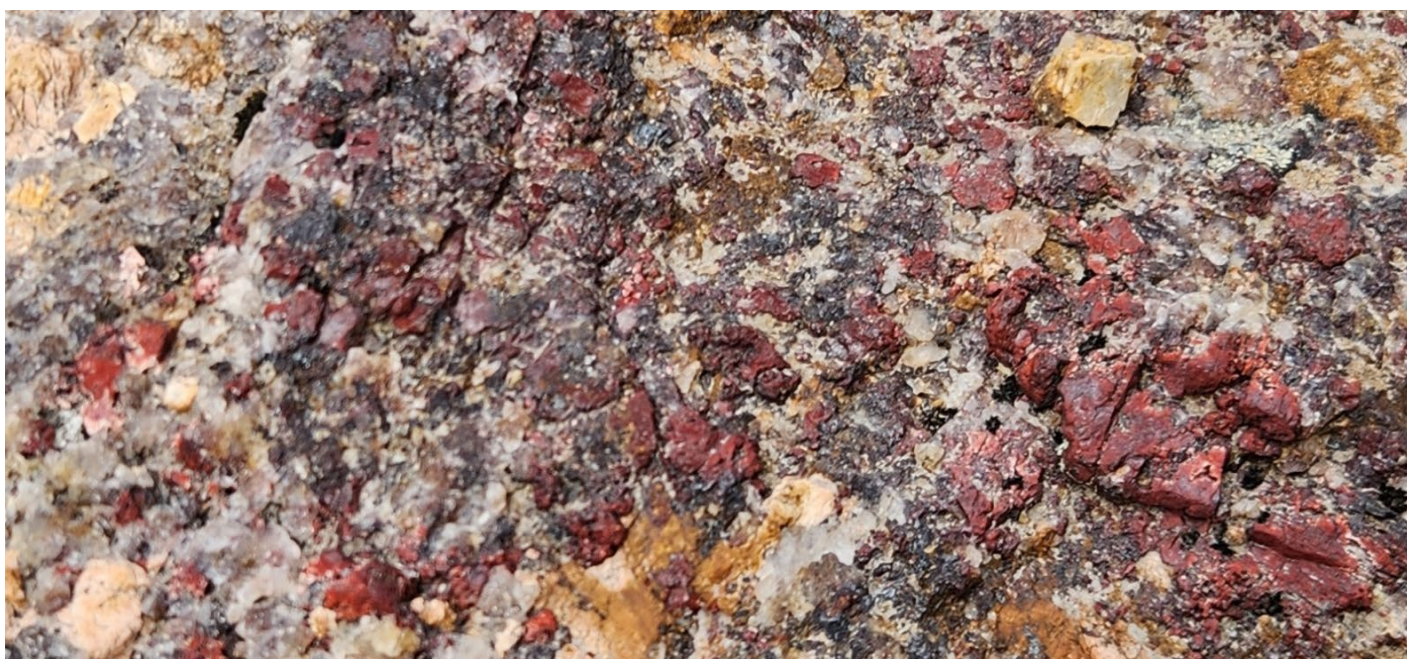
Figure 2. Close-up photograph of red-coloured mineral grains visually interpreted as eudialyte-like minerals hosted within coarse-grained alkaline granite. The minerals occur as scattered grains and irregular aggregates within the host rock. The visual interpret
