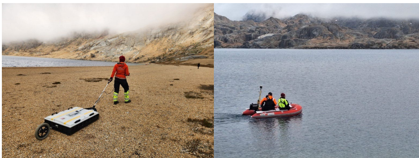
Figure 18. GPR and Bathymetrical surveys being completed at the Blue Lagoon Project.
