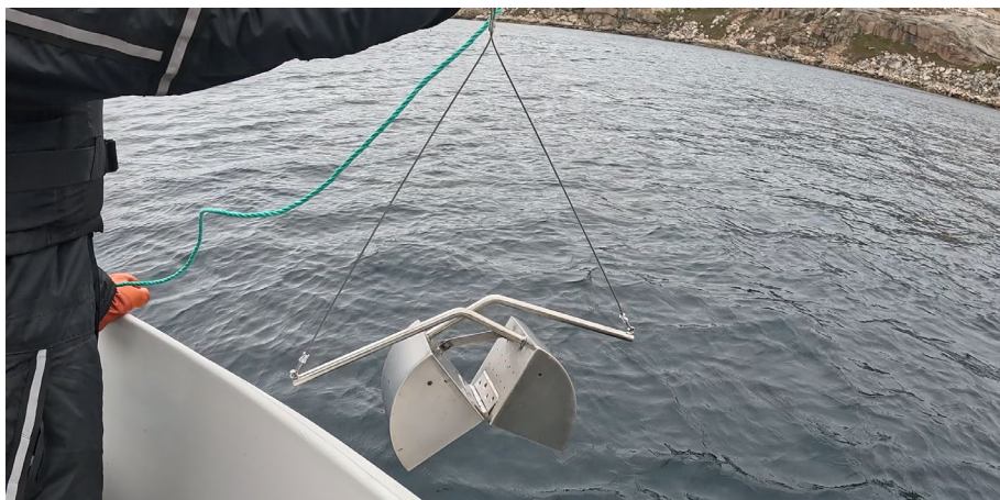
Figure 19. Van Veen grab sampler used during the 2026 exploration program to collect sediment samples from the Blue Lagoon and selected nearshore marine locations.
