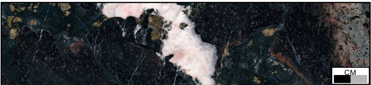
Figure 8: SPD056 – 254.4m, 5.14 g/t Au . Andesite with hematite dusted feldspars and patchy albite-hematite alteration showing a chlorite-pyrite-carbonate-chalcopyrite crackle breccia and late carbonate-pyrite vein.
