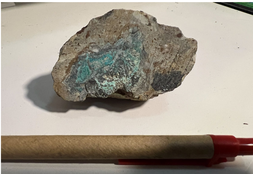
Figure 2. Sample MR0011 showing green malachite and dark grey galena mineralisation in carbonate host rock with darker brown iron-carbonate fragments.
