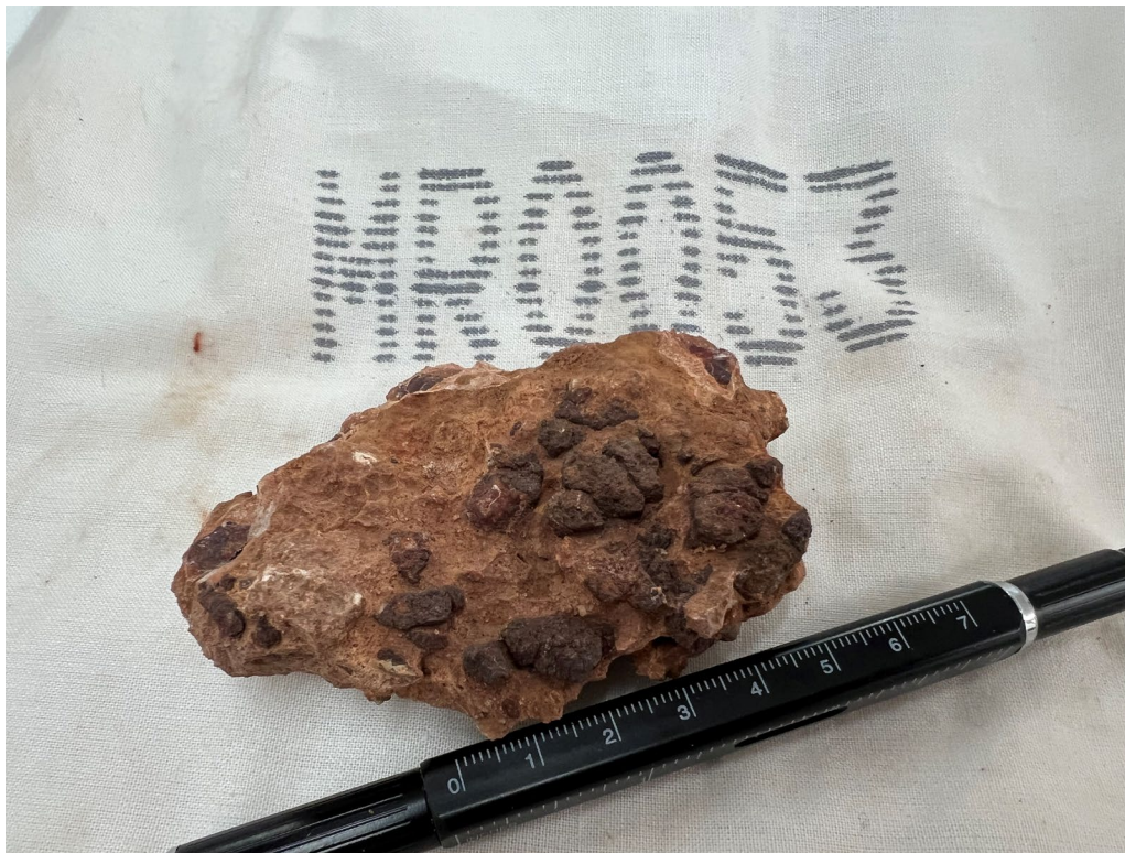
Figure 3. Sample MR0013 (originally MR0053) showing weathered breccia material with dark brown iron-carbonate nodules.
