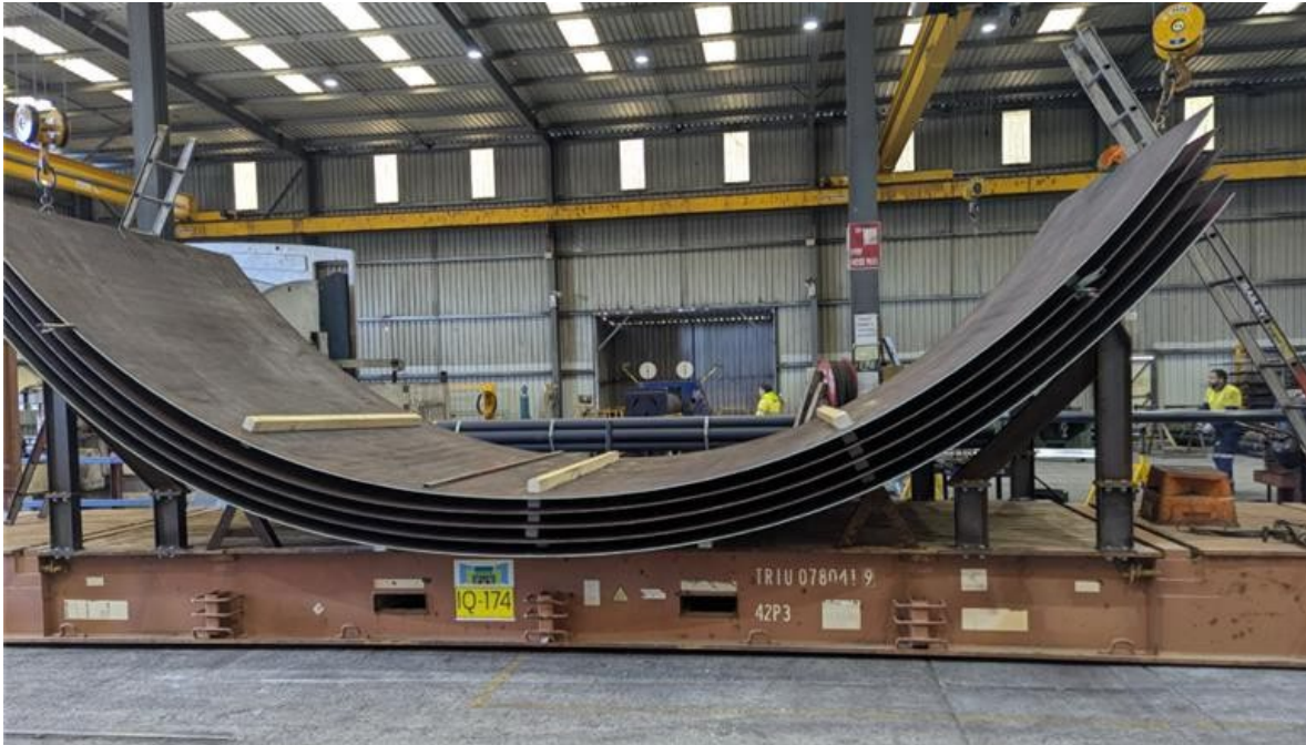
Figure 4 – CIL tank steel rolled in preparation for transport
