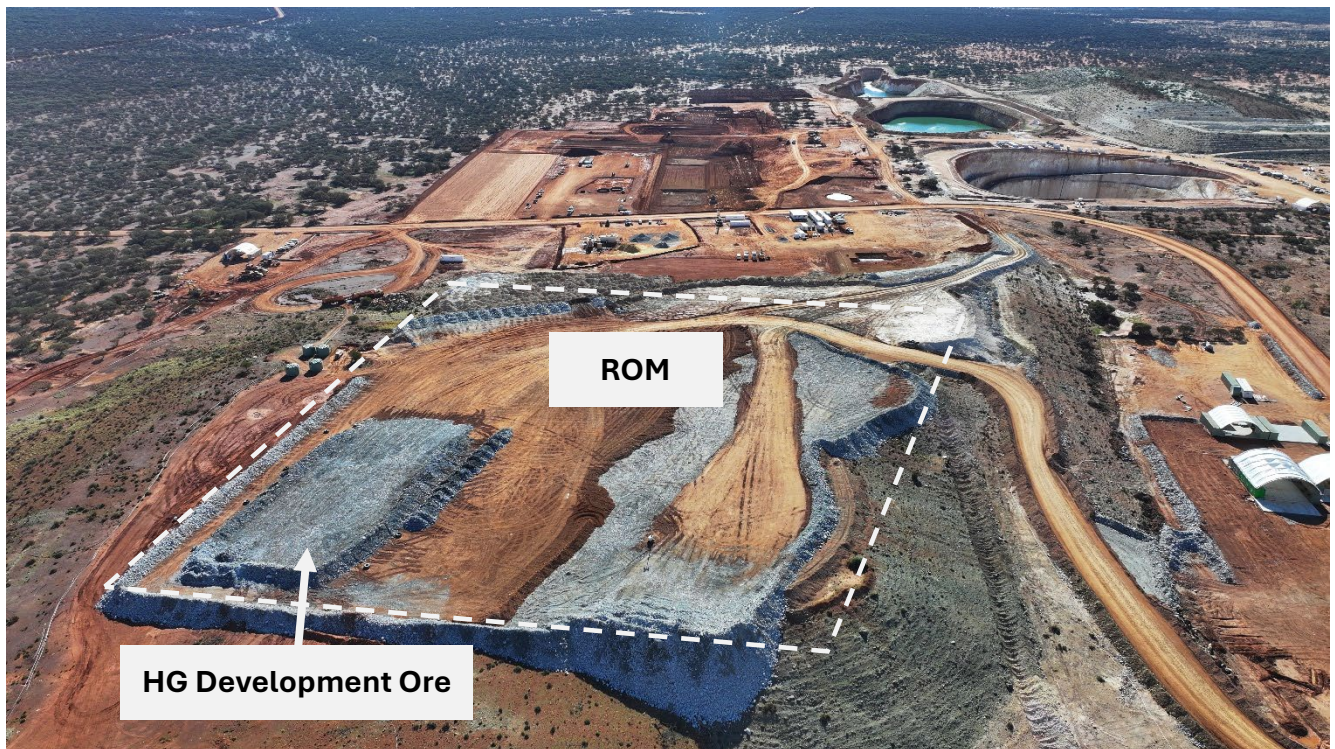
Figure 8 – Ore stockpile build on main ROM
