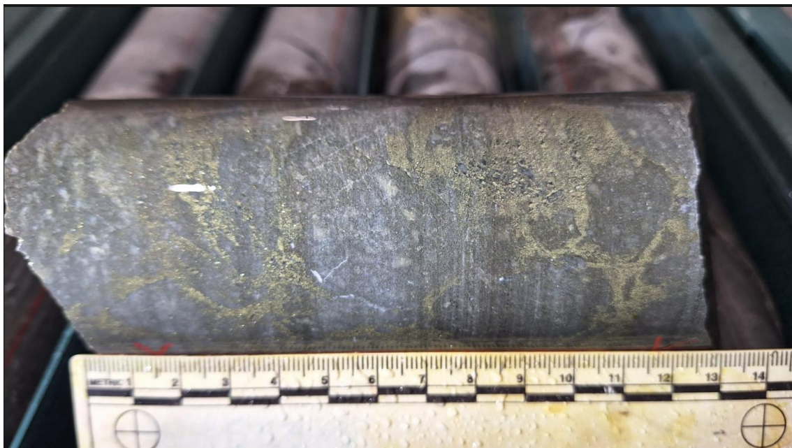
Image 1 - Strongly pyritic 50% at 1153.7m
