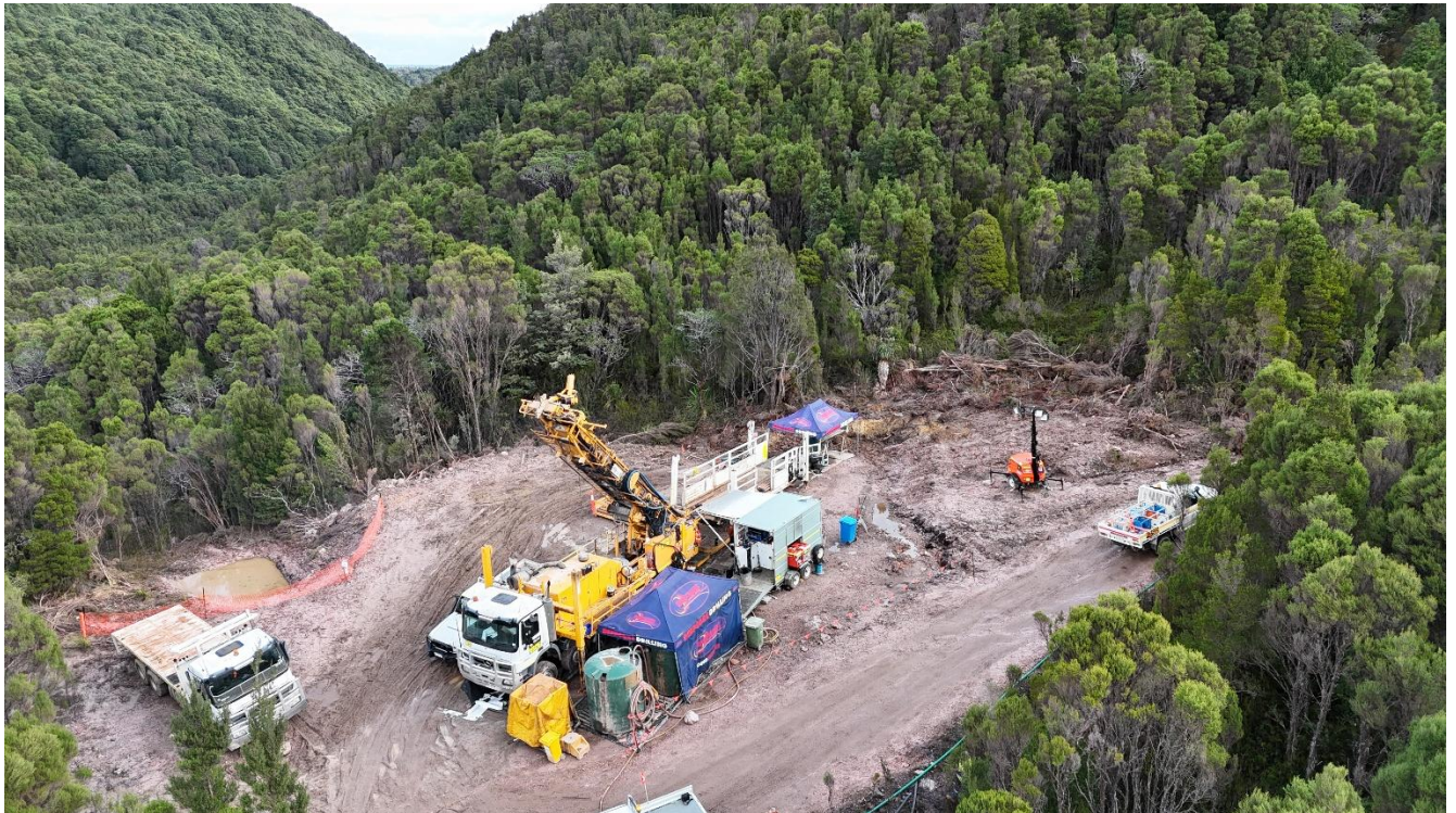
Image 5 - Photograph showing diamond rig onsite drilling the Zig Zag West anomaly
