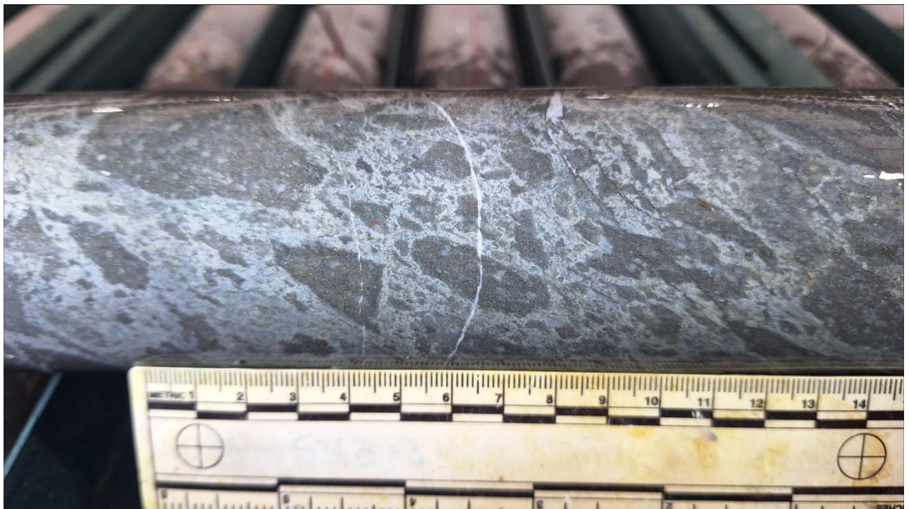
Image 3 - Pyritic rhyolitic breccia 15-20% py at 1113.5m
