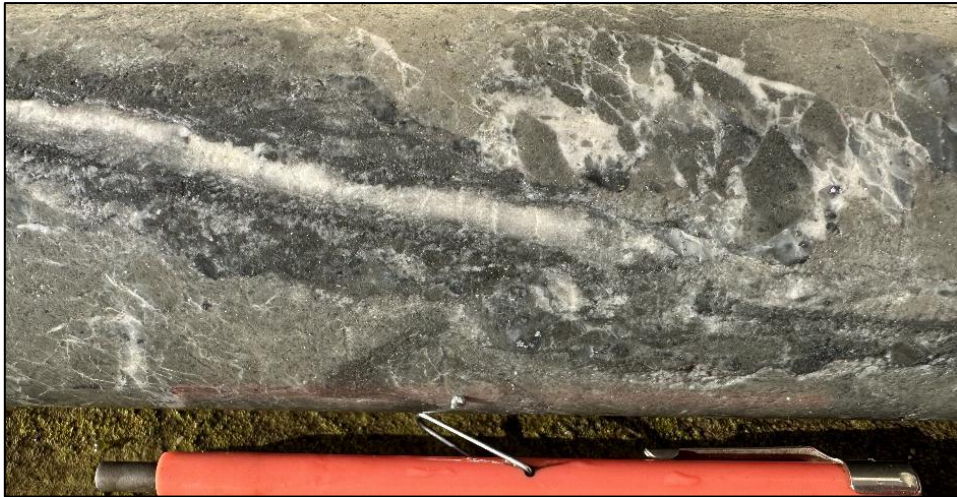
Early pyrite then later carbonate fracture-fill veins. 447.0m.
