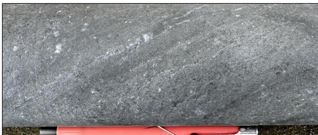
Laminated and/or veined tuffaceous sandstone. 420.2m.
