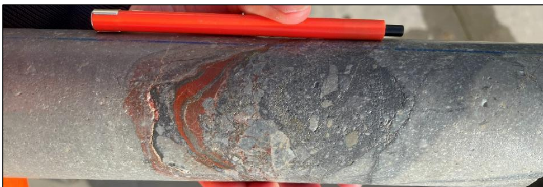
Hematite rimming pyrite vein, as breccia infill and in selvage of breccia vein in sericite+illite altered Andesite Breccia. 140m.
