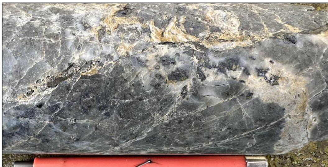
Quartz+carbonate vein with galena, honey-coloured sphalerite and chalcopryite. 415.0m.
