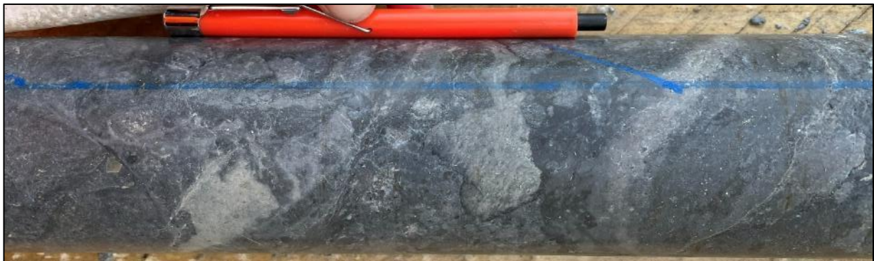
Wispy juvenile dacite clasts in Andesite-Dacite breccia. 377.2m.
