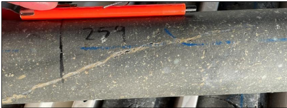
Quartz + carbonate + siderite vein overprinting earlier pyrite veinlet (with sericite selvage) in weakly quartz + sericite + pyrite altered porphyry andesite. 259m.
