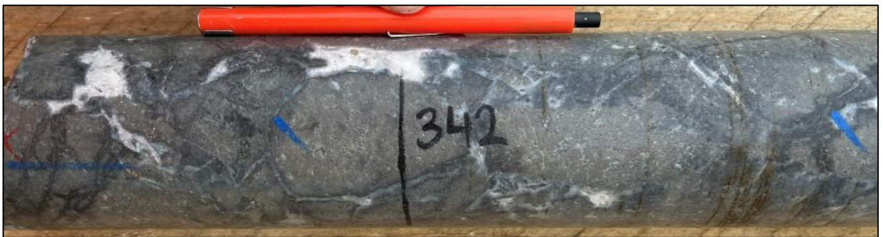
Quartz vein with later carbonate + sphalerite (honey coloured) + chalcopryite + galena and (?) trace black sulphides in andesite breccia. 342m.
