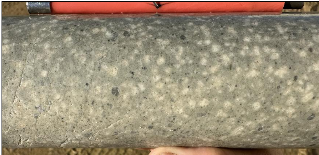
Late quartz+feldspar porphyry. Weak to moderate pervasive clay. 499.2m.
