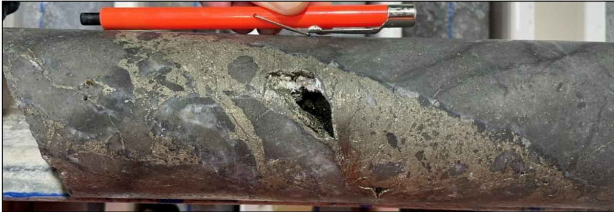
Breccia vein with pyrite overprinting chalcedony with significant galena + sphalerite (honey coloured) + chalcopyrite. 398.5m.
