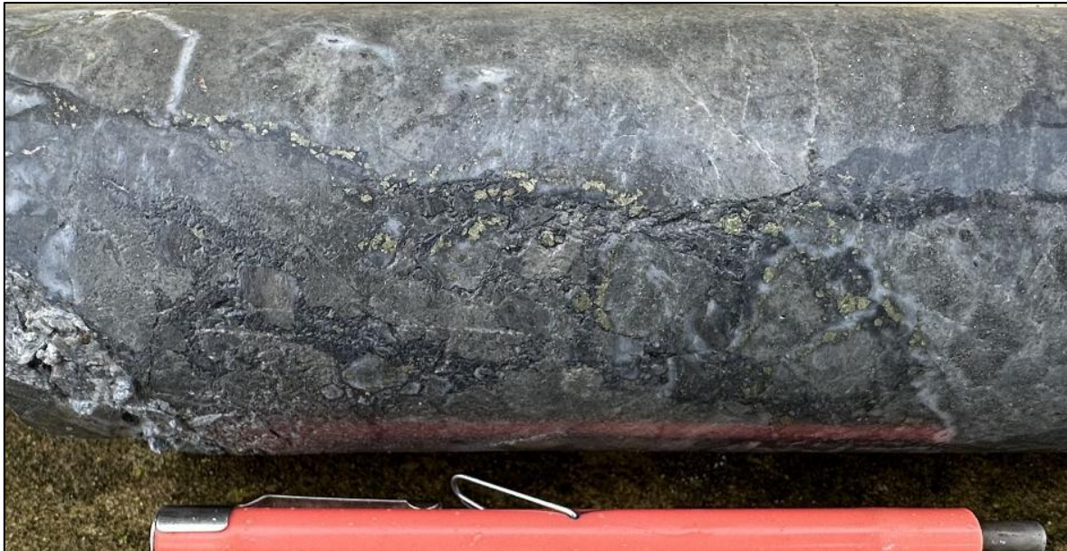
Trail of chalcopyrite blebs in polymictic breccia. 434.6m.
