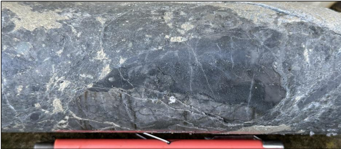
Silicified quartz+pyrite-altered clast within polymictic breccia. 430.4m.
