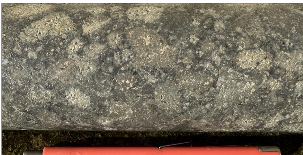
Andesite-clast breccia. Weak to moderate pervasive clay. 464.1m.
