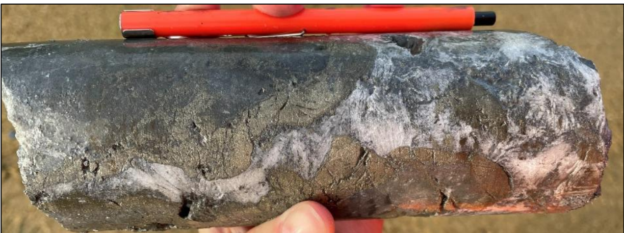
Breccia vein with massive pyrite infill and later quartz + bladed carbonate (replaced) infill with trace black sulphides within andesite. 234.2m.
