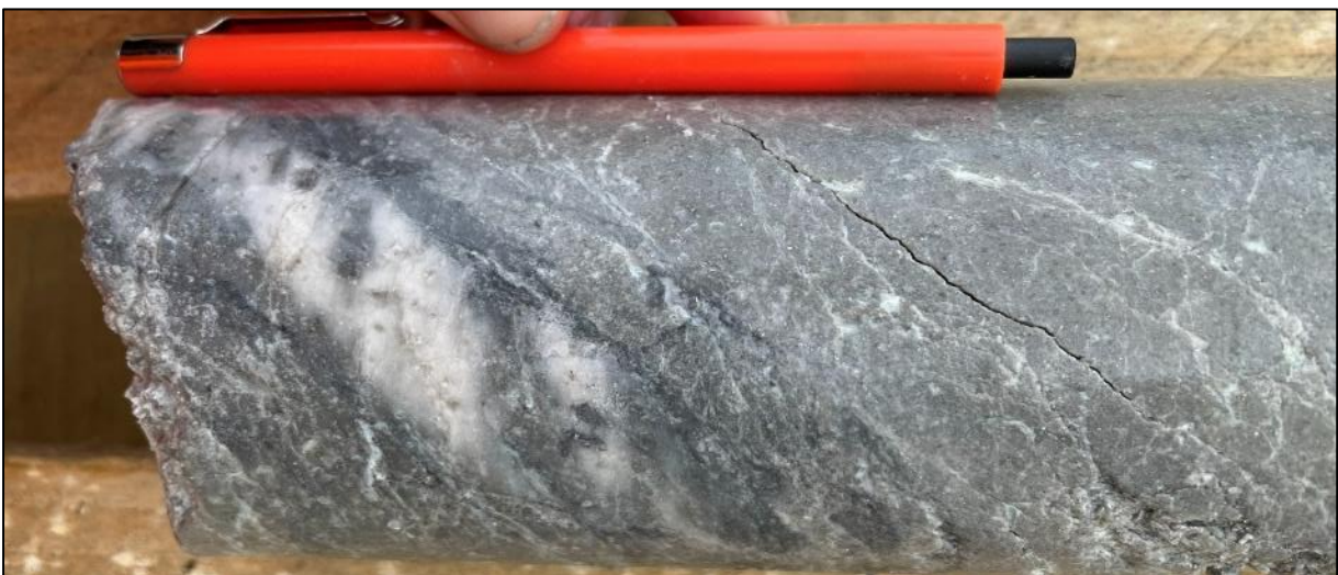
Quartz vein with ~5mm galena crystals in fractured andesite. 366.9m.
