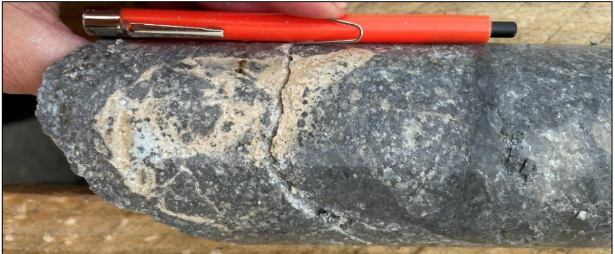
Siderite with sphalerite (honey coloured) and sericite within Andesite-Dacite breccia. 372.3m.
