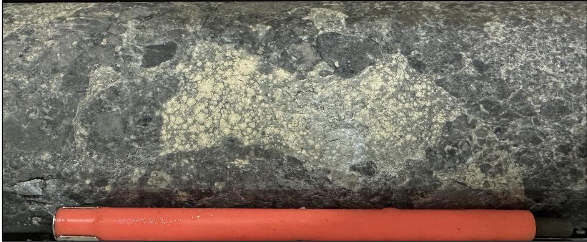
Ragged, yellow ankerite-altered andesite clast. 427.1m.
