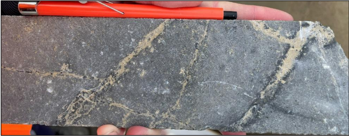
Siderite vein with galena + sphalerite + (?)black sulphides in illite+quartz altered andesite. 332.8m.
