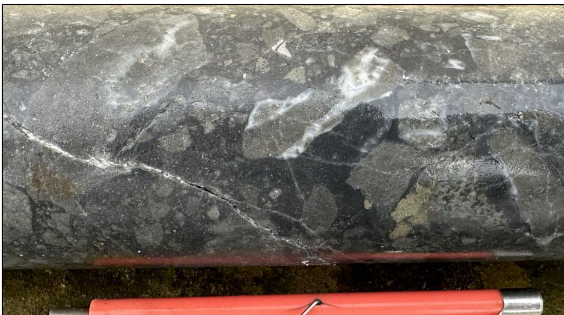
Ragged clasts with quartz+carbonate veins in polymictic breccia. 434.15m.
