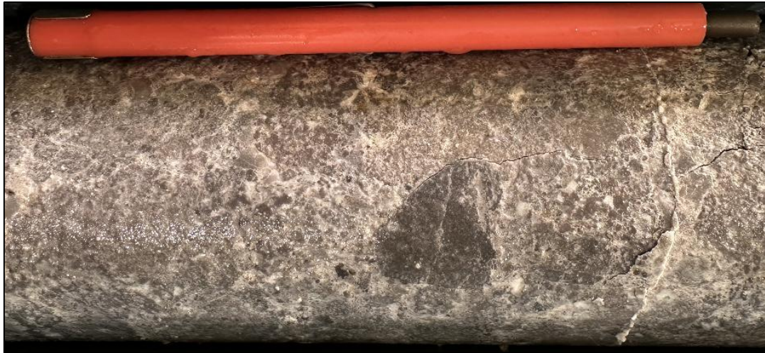
Matrix-supported andesite-clast breccia. Strong pervasive clay. 490.8m.
