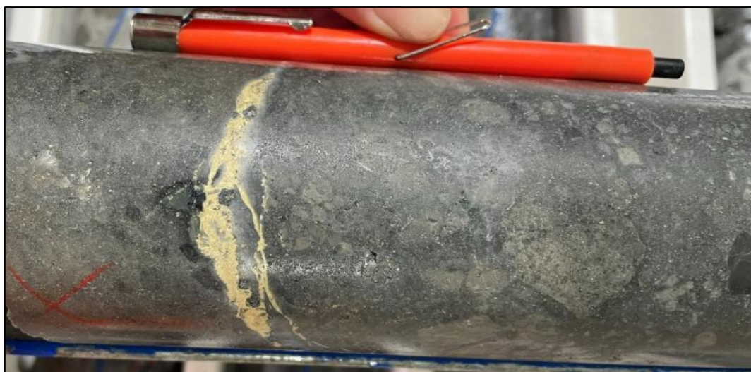
Chalcedonic quartz+carbonate vein with siderite + galena + honey-coloured sphalerite infill within Andesite clast breccia. 408.9m.
