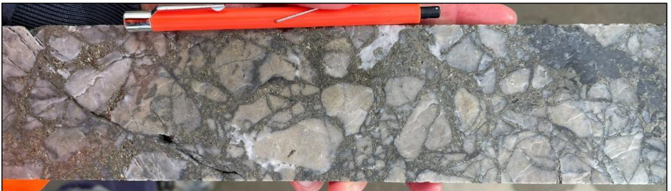
Strongly silicified + sericite altered andesite clast breccia with pyrite cement (includes ~0.5% galena). 173m.
