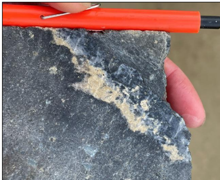
Quartz + Siderite vein with galena + sphalerite + (?) black sulphides in illite + quartz altered andesite. 332.5m.
