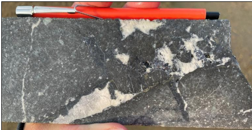
Quartz+carbonate+galena+sphalerite (honey coloured) within quartz+pyrite altered andesite breccia. 220.3m.
