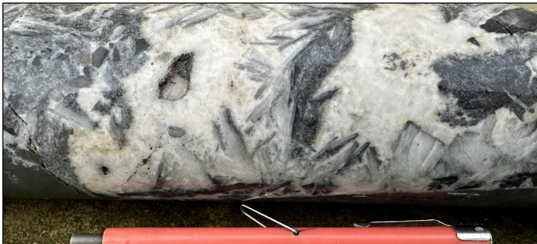
Quartz+carbonate+?adularia open-space fill. 437.4m.
