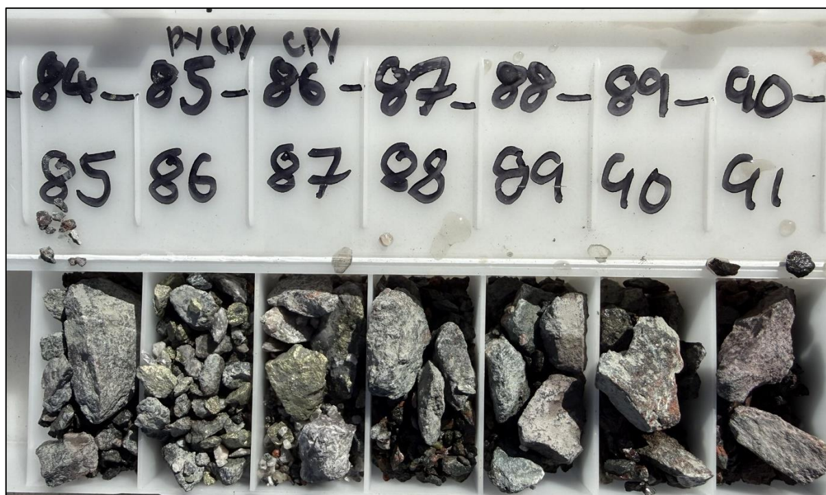
Figure 2 Representative example of sulphides (chalcopyrite ± pyrite) visually identified in RC drill chips. [Hole 26MIE-005, @ 84-91 m downhole; Ardmore North.] Image unedited; colours not enhanced; Downhole depths annotated on tray are in metres. Visual identification only; not confirmed by assay and not indicative of grade, width or continuity. Depth range shown is the extent of the chip tray photographed; sulphides occur at points within it, not as a continuous interval.
