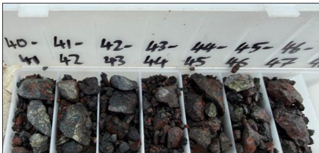
Figure 1 Representative example of sulphides (chalcopyrite ± pyrite) visually identified in RC drill chips. [Hole 26MIE-011, @ 40-47m m downhole; Ardmore North.] Image unedited; colours not enhanced; Downhole depths annotated on tray are in metres. Visual identification only; not confirmed by assay and not indicative of grade, width or continuity. Depth range shown is the extent of the chip tray photographed; sulphides occur at points within it, not as a continuous interval.
