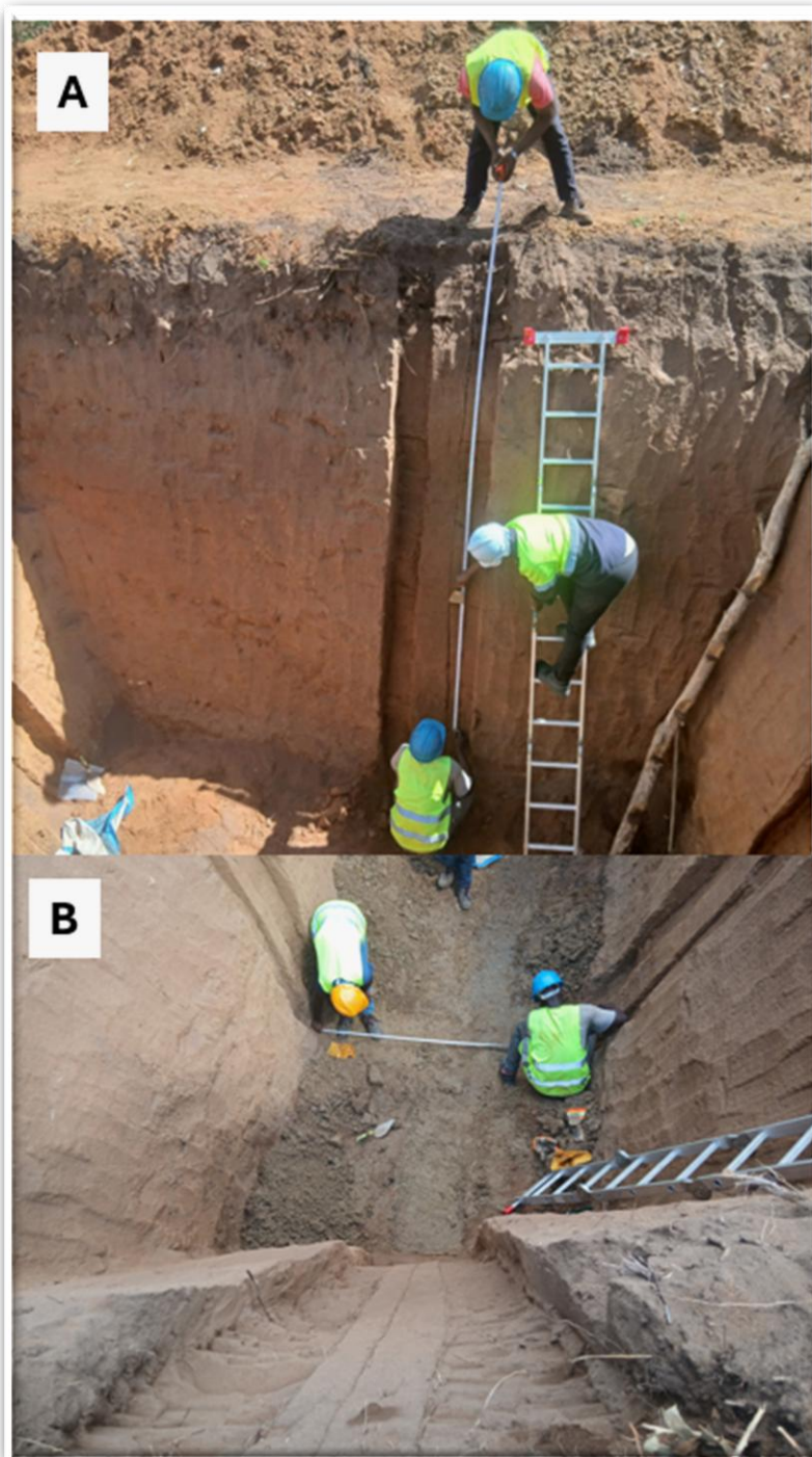
Figure 3: A) Lithological sampling taking place at Pit 3; B) sampling taking place of the subcrop at the base of Pit 3.
