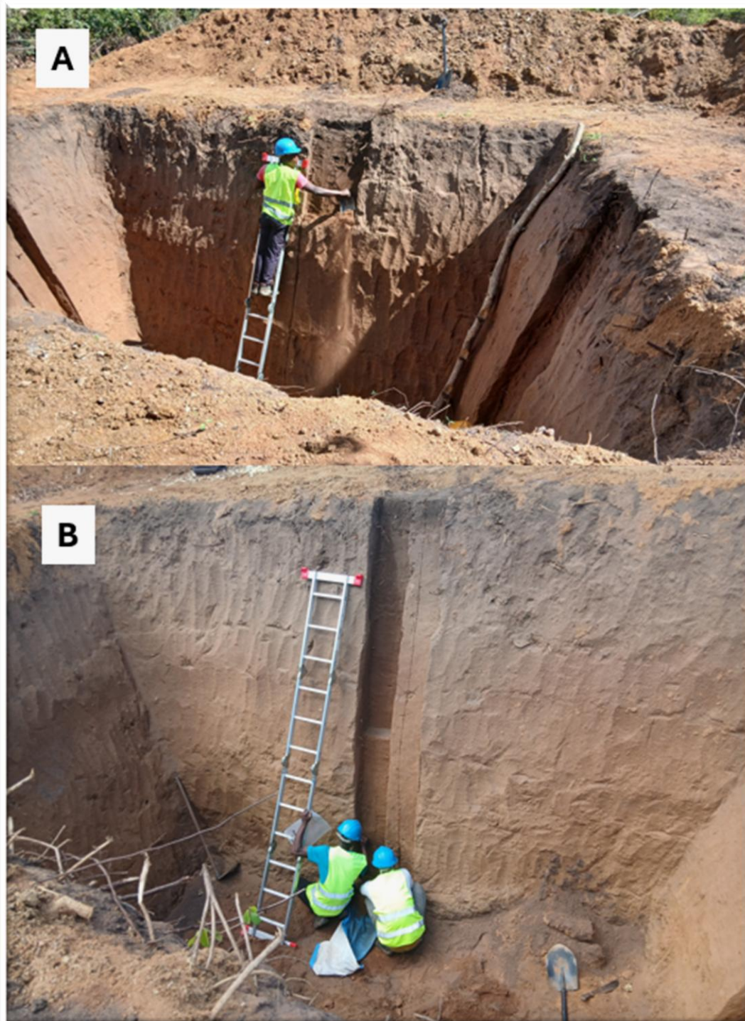
Figure 2: A) Sidewall being cleaned at Pit 3 for sampling; B) Sampling of the 1m interval samples taking place at Pit 3; C) View of one of the sidewalls in Pit 3 of the 1m interval and lithological sample cuts that have been completed; and D) sampling taking place of the subcrop at the base of Pit 3.
