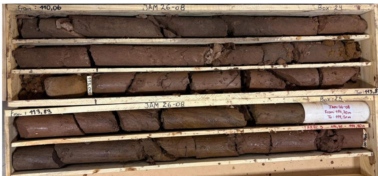
Figure 3. Core sections and core taken for porosity testing at 113.83m.
