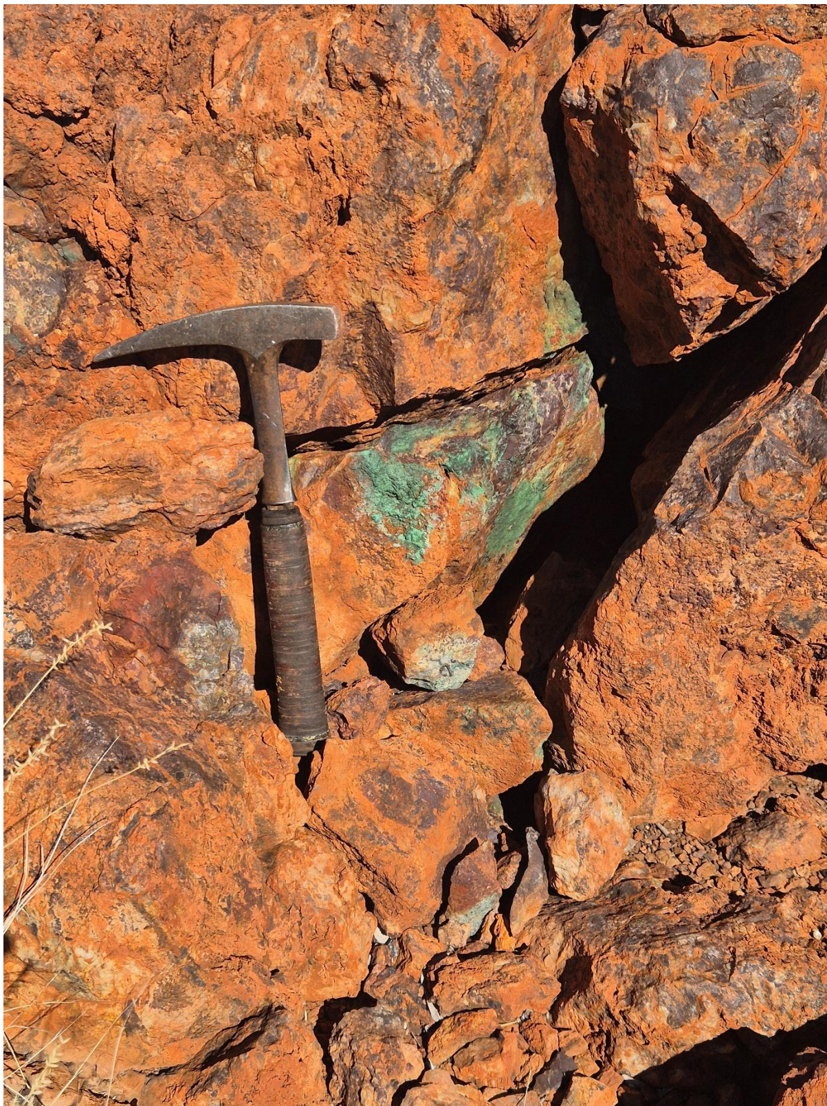
Figure 3: Malachite and chrysocolla within gossan (Sample TM10512).
