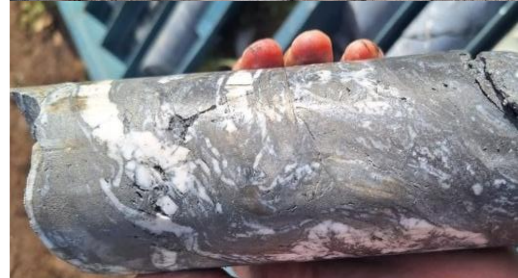
Photograph of core from DD25ZOP014 which returned 24.3% Sb and 7.6g/t Au
