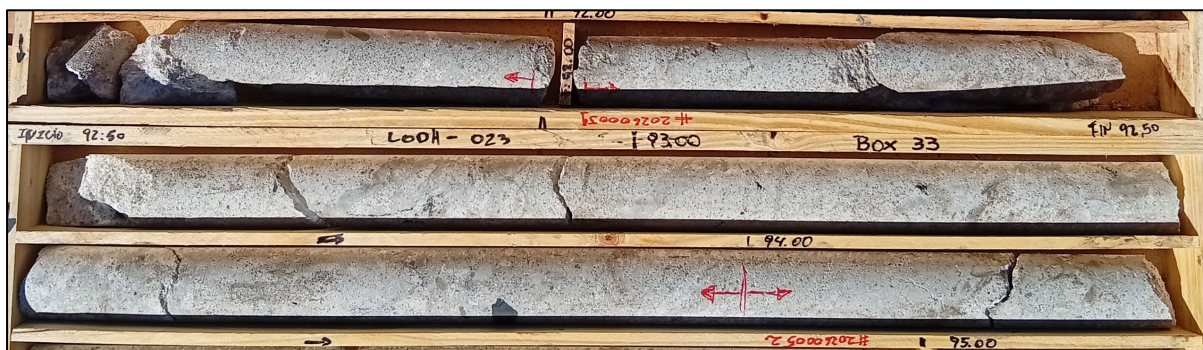
Figure 5: Drill core between 92-94m which provided 2m @ 5.21g/t Au, 0.47% Zn and 3.81g/t Ag.
