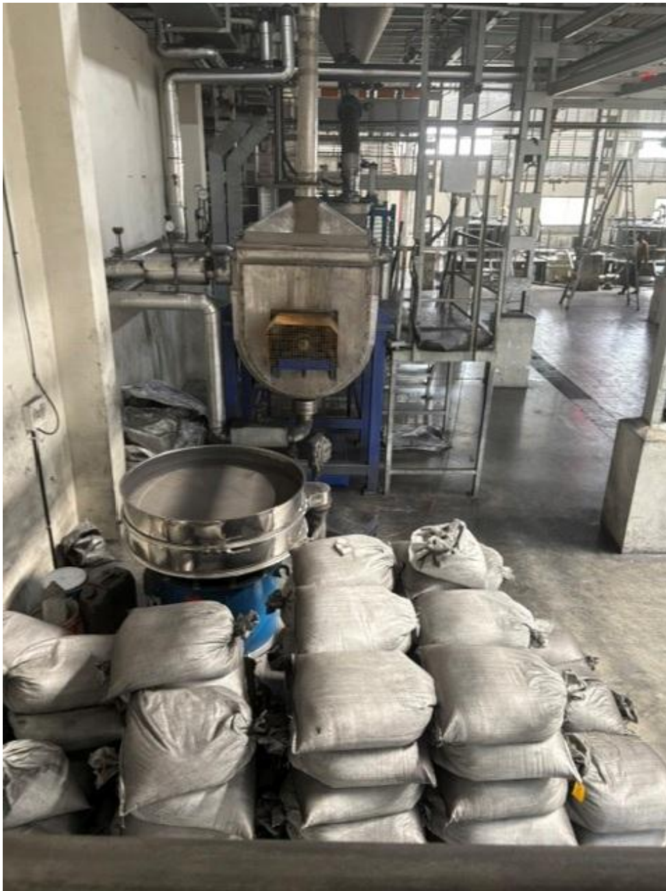
Figure 2 – final screening of finished product on site 22 June 2026
