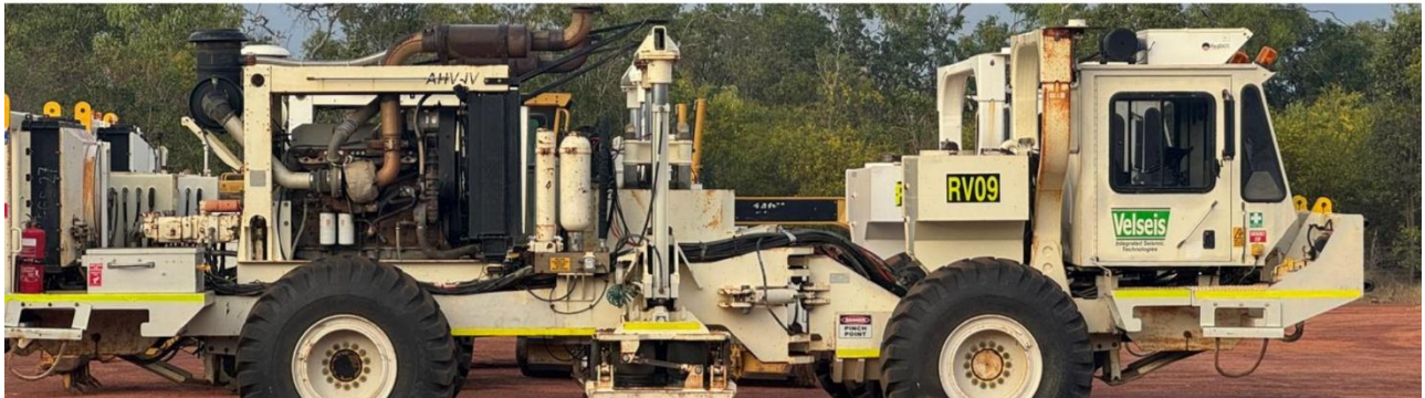
Vibroseis truck used for generating seismic waves to map underground geological structures
