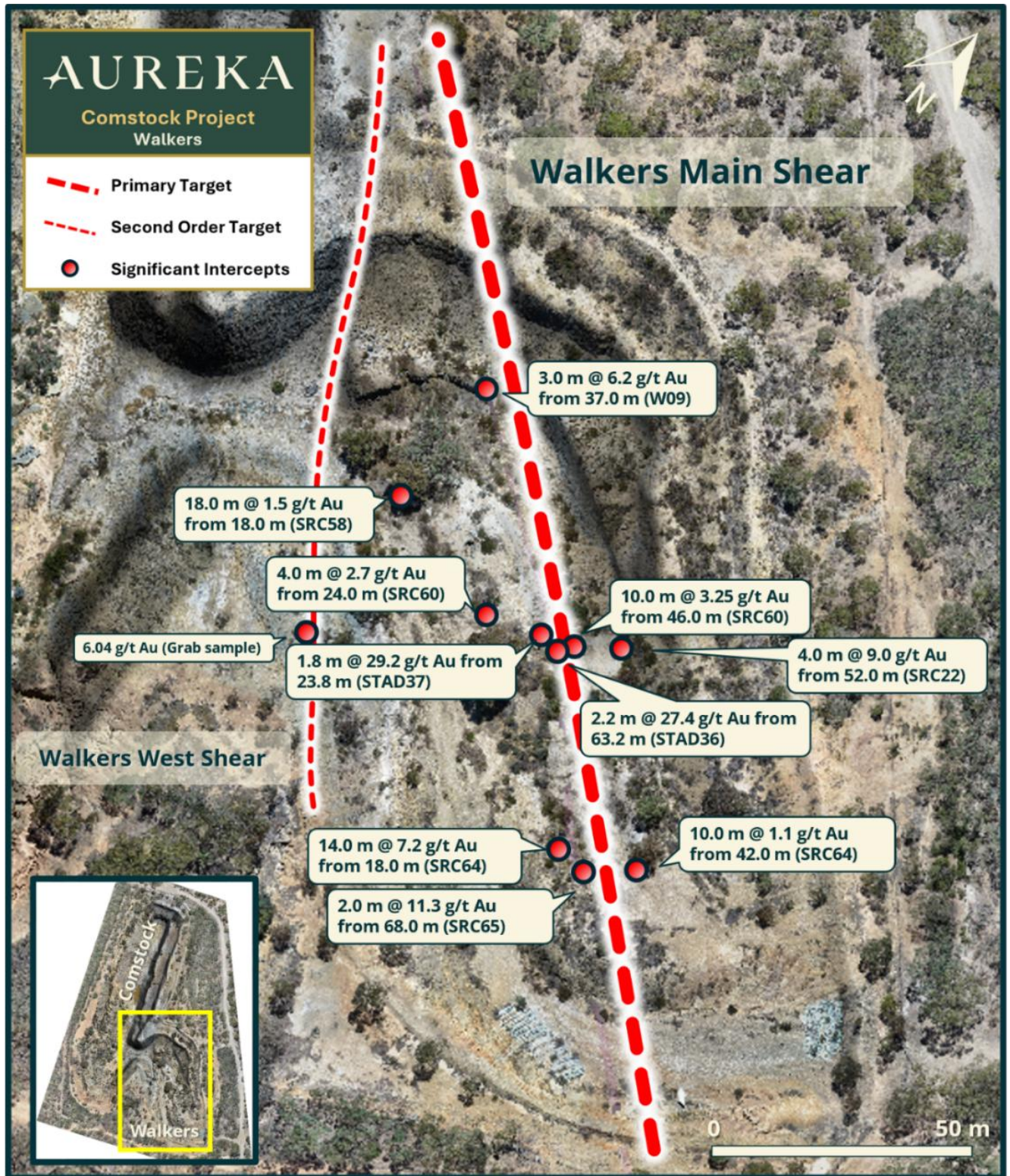
Figure 4 – Plan View of the Walkers sub-pit and the Walkers main Shear with legacy drill intercepts projected to pit floor surface 16 . Historical legacy drilling has been re-published with JORC Tables in this release refer Appendix A and B.
