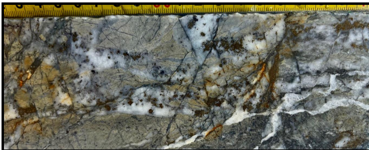
Figure 3 - Hole L1MP5DD003 (99.8m) - Drill core sample with multi-phase mineralising events within silicified rhyolite porphyry
