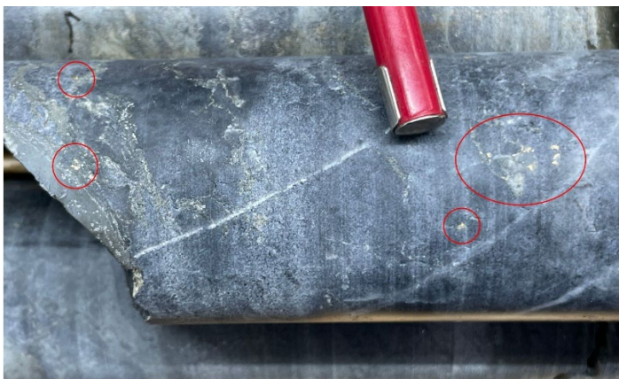
Figure 4 (LHS): Photo of core showing visible gold grains in 20cm smoky quartz vein hosted in sulphide, chlorite-carbonate altered wacke, 187.90m, BO-25-27. Scale unit is in cm.
