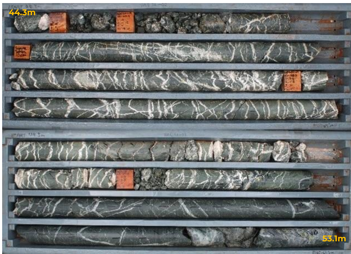
Figure 5. HDD26-01 – showing intense quartz-carbonate veining occurring within at least two phases of alteration. Depth 44.3m to 53.1m
