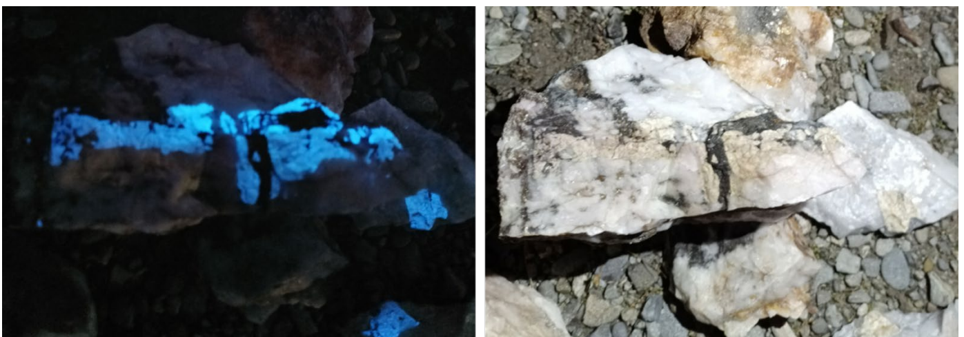
Figure 1 – Scheelite-bearing quartz float sample A1411 at Granite Creek under plain light (right) and ultraviolet light (left). The intense blue-white fluorescence under UV illumination highlights the distribution of scheelite within the quartz sample. A1411 returned 8.01% WO 3 .
