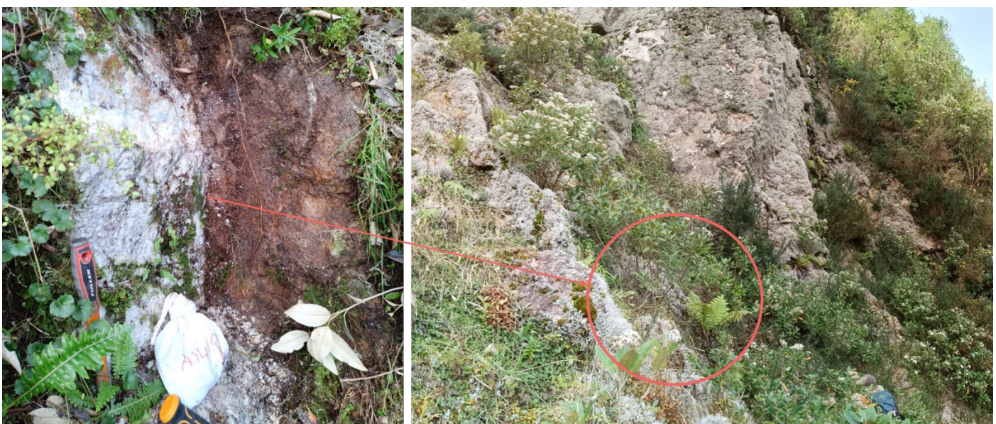
Figure 3 – Left - Quartz-scheelite vein exposure at Granite Creek, New Zealand. Channel sample A1419 was collected perpendicular to the vein across its 0.41 m true width and returned 16.63% WO 3 . The adjoining 0.20 m footwall sample A1420 returned 3,820 ppm W. Geological hammer shown for scale. Right. Location of channel sample.
