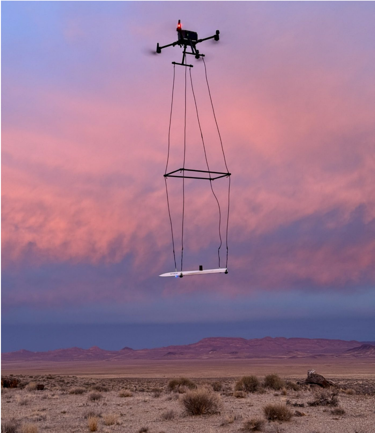
Figure 1: Drone commencing the magnetic survey at Iron Butte.
