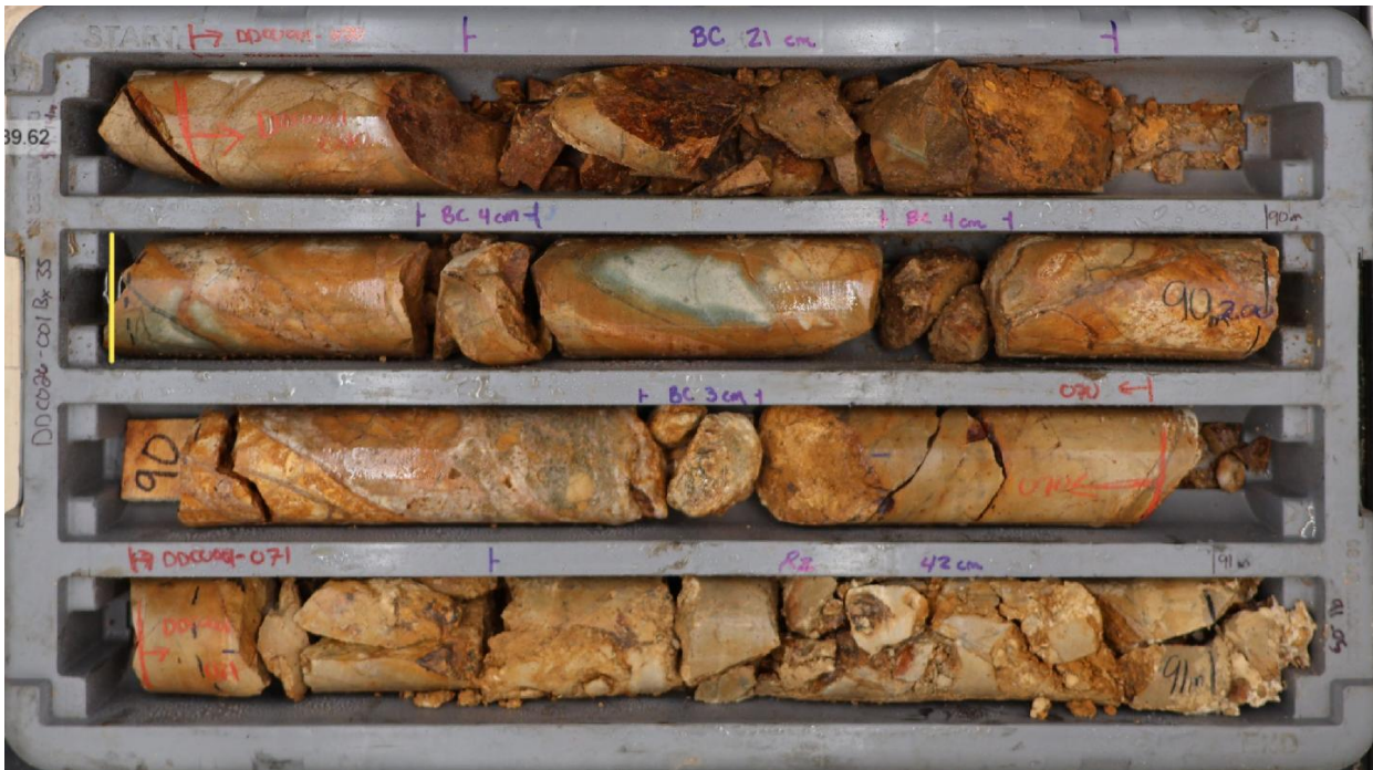
Figure 2. Representative drill core from DDCO26-001 (89-91m). Near-surface oxidised material: note argillic alteration, quartz-chalcedony veining, and vugs with iron staining after oxidised sulphides. Visual observations only; not a proxy for grade.
