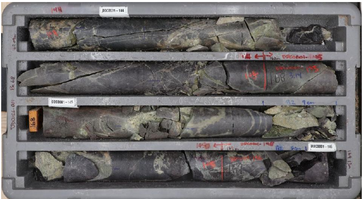
Figure 3. Representative drill core from DDCO26-001 (167-169 m). Deeper fresh (unoxidised) material: note lower alteration intensity, quartz-chalcedony veining, very competent without iron staining as sulphides are unoxidised. Visual observations only; not a proxy for grade.
