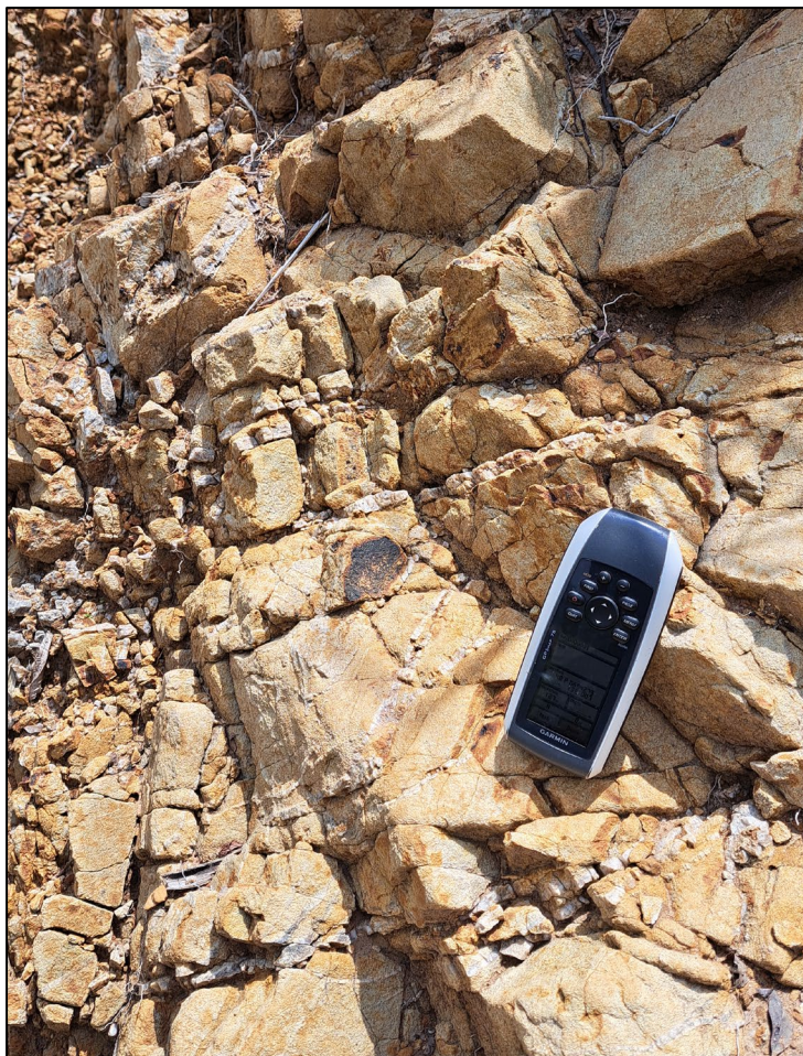
Figure 3: Stockwork veins hosted in altered diorite at Rohav Mountain Prospect. Veins exposed in recent extensions to alluvial artisanal workings in a creek cutting through the diorite intrusion. Assays for rock chip sampling of these veins are pending.
