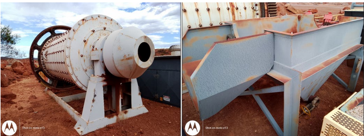
Figure 12: Ball Mill and discharge chute
