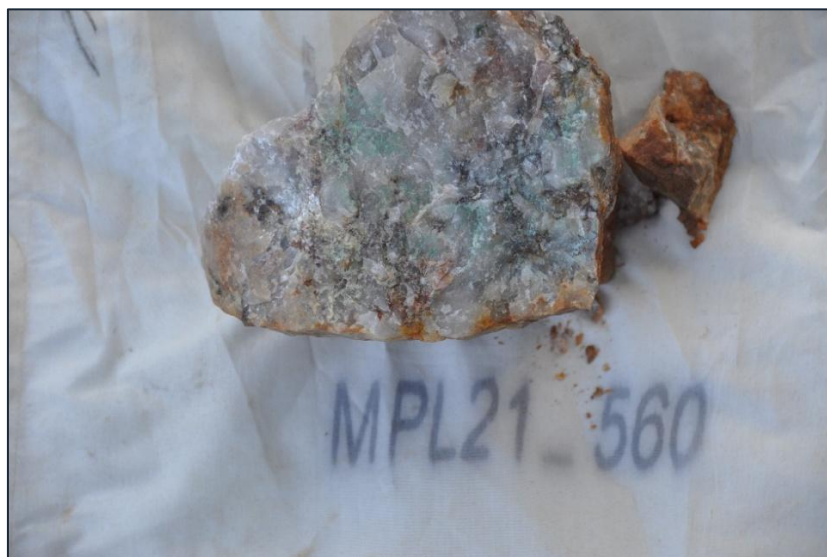
Figure 3. In-situ sample from the Makinsons Mine area (MPL21_560) comprising quartz vein containing coarsely disseminated malachite, hematite, chalcocopyrite, bornite, and wolframite.
