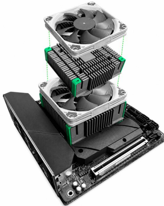
Figure 2: Render image of prototype design of VHD Mini-ITX motherboard heat sink
