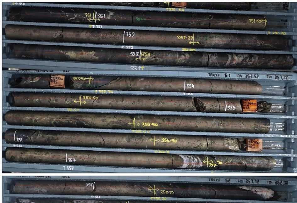
Figure 1: ~6.65m interval of massive and semi-massive sulphides overprinting quartz veining from 351.2m, comprised of pyrrhotite (60%) and semi-massive chalcopyrite (15%) and pyrite (5%). True width of the interval is estimated to be approximately 50% of the visually logged intercept length.
