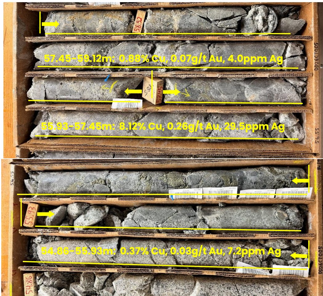
Figure 1: High grade copper mineralisation between 54.86–59.12m down hole DD26CT005.
