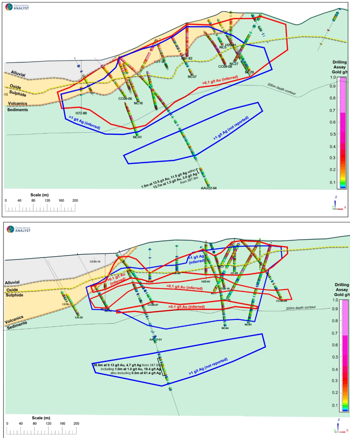
Figure 4: Central cross section (above) and southern cross section (below) showing geology, base of weathering (yellow dash), alluvial (grey dash) in relation to the gold-silver inferred wireframes (red) and silver-only wireframes (blue). Note: a portion of the lower silver-only wireframe is below 200m depth and therefore not reported as part of the MRE but represent exploration potential. For cross section locations see Figure 5.
