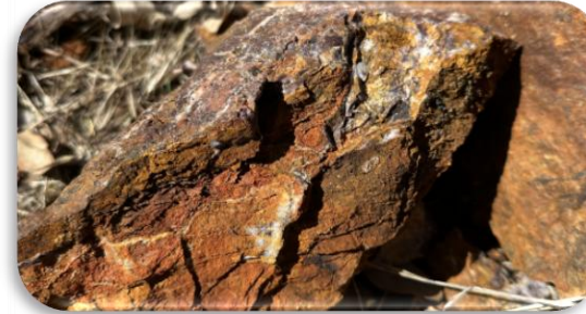
Gossanous and quartz veined volcanic sandstone 2.16 g/t Au (sample 8864-002)
