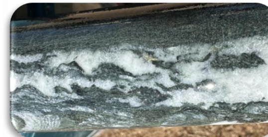
Quartz + pyrite + chalcopyrite veined volcanic sandstone (PORD003 709m)
