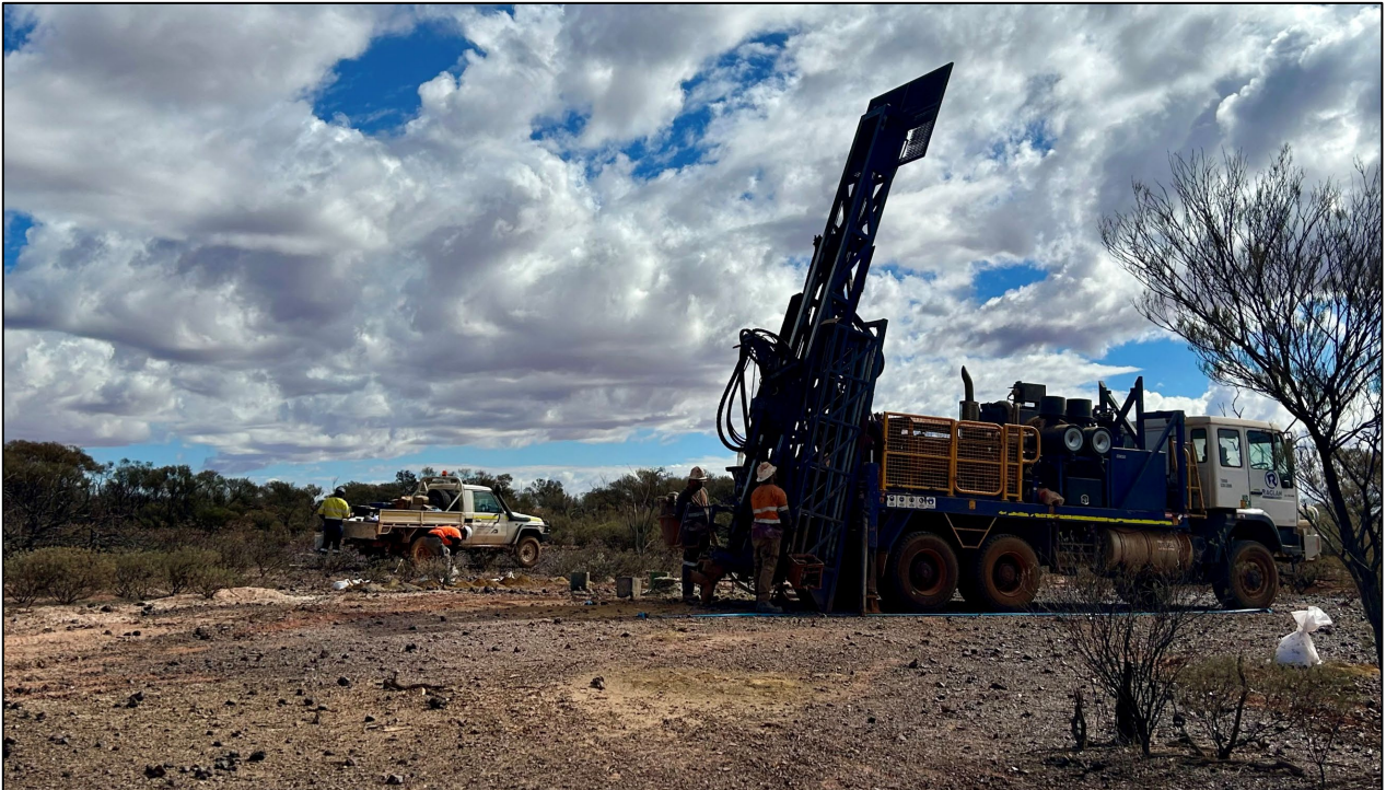
Figure 2: Air core drilling at the Diorama Copper-Gold Target.
