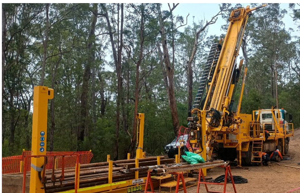
Figure 1. Diamond drill rig set up at the Emu Copper-Gold Prospect.
