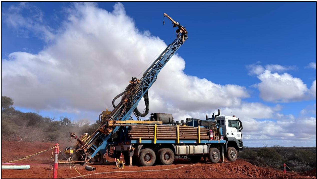
Figure 1: RC drilling first hole at Brunswick Hill trend.
