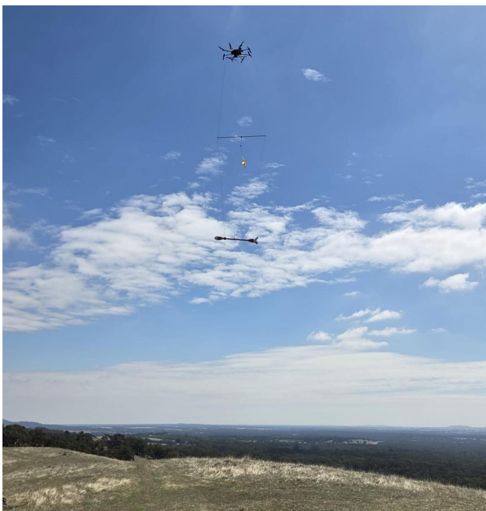
Figure 4: Drone and connected magnetometer actively collecting data over Aureka's Irvine Project.
