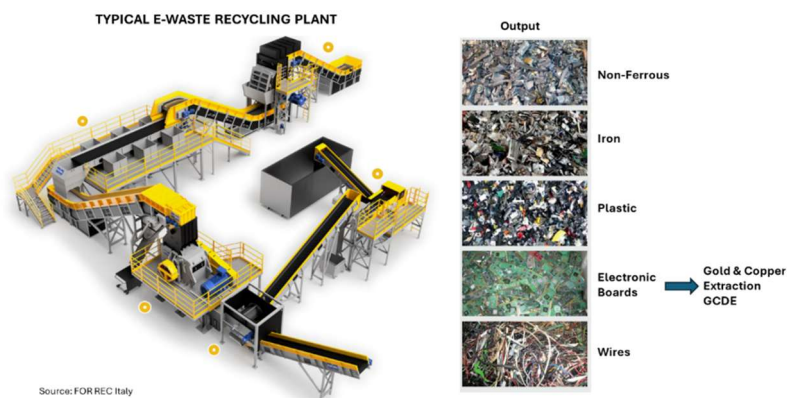
Figure 1 – E-Waste available from market processed through typical recycling plant
