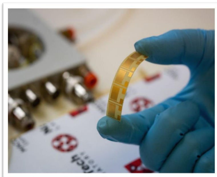
Figure 1: Nanosensor strip demonstrating pathways to device integration and scalable form factors such as E-skin applications
