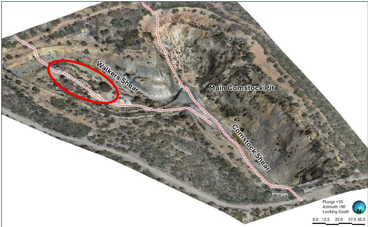
Figure 6 – View of the high-accuracy LiDAR and photogrammetry of the Comstock open-cut pit – looking towards the South (azimuth 18). Red circle highlights current drill target area for infill diamond drilling now underway.
