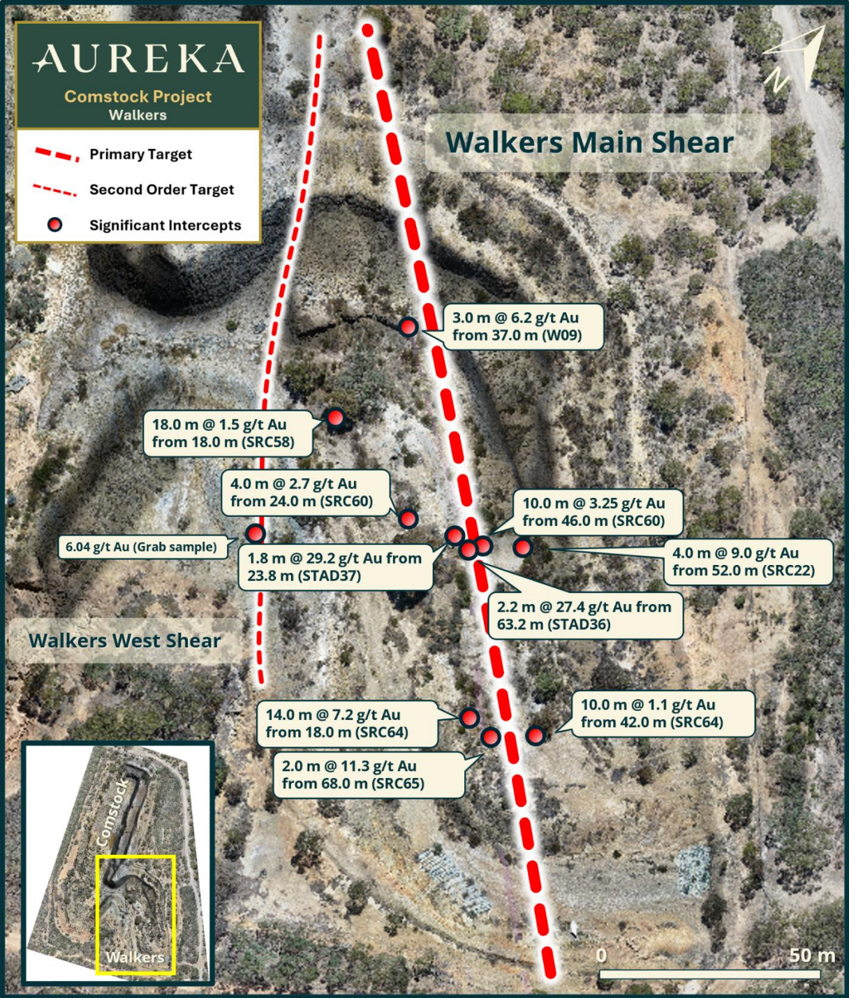
Figure 2 – Plan View of the Walkers sub-pit and the Walkes main Shear with legacy drill intercepts projected to pit floor surface. Historical legacy drilling has been re-published with JORC Tables in this release refer Appendix A&B.
