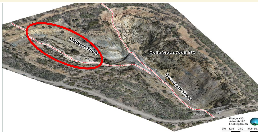
Figure 1 – View of the high-accuracy LiDAR and photogrammetry of the Comstock open-cut pit – looking towards the South (azimuth 18). Red circle highlights drill target area for the 6-week infill diamond drilling program now underway.
