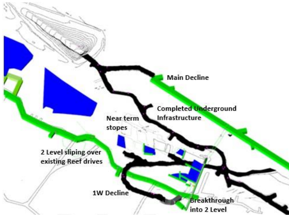
FIGURE 2: 1 WEST BREAKTHROUGH PROVIDES ACCESS TO ESTABLISHED 2 LEVEL STOPES
