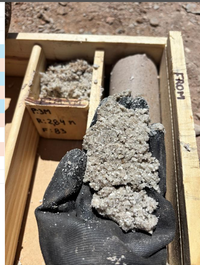
Sample from 284m level showing porous sands with 295pp lithium
