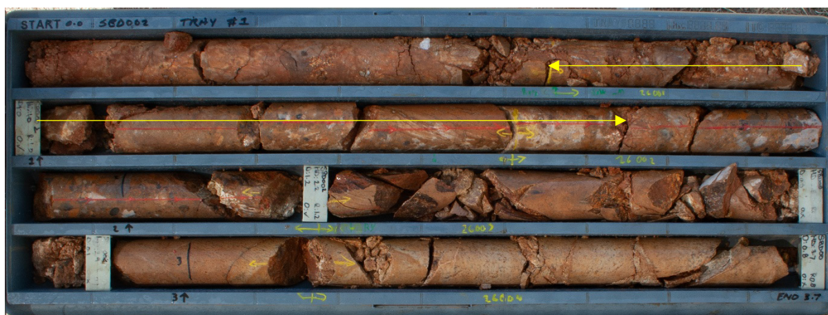
Figure 10: SBD001 core example. Yellow arrow indicates section between 0.6-1.6m which yielded 0.69g/t Au.
