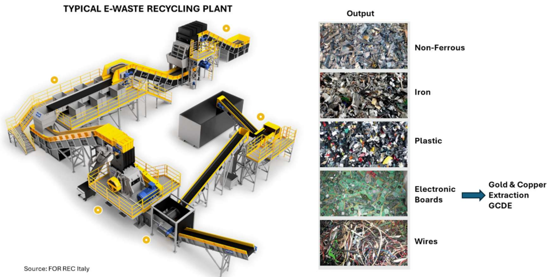
Figure 3 – Typical E-Waste recycling plants separating electronic boards
