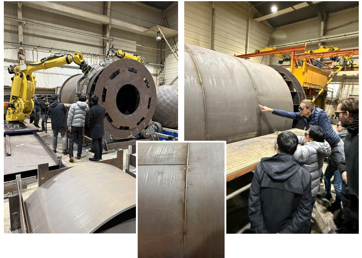
Robotic Cell: Plate handling, mounting, tack welding and seam welds
