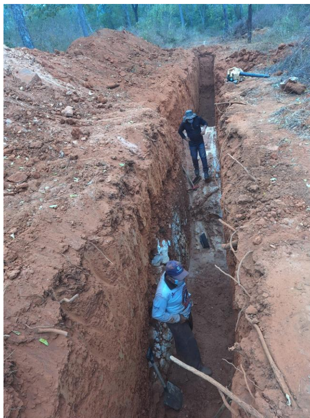
Figure 1: Channel sampling underway at Trench TR01, Mauricio Target.
