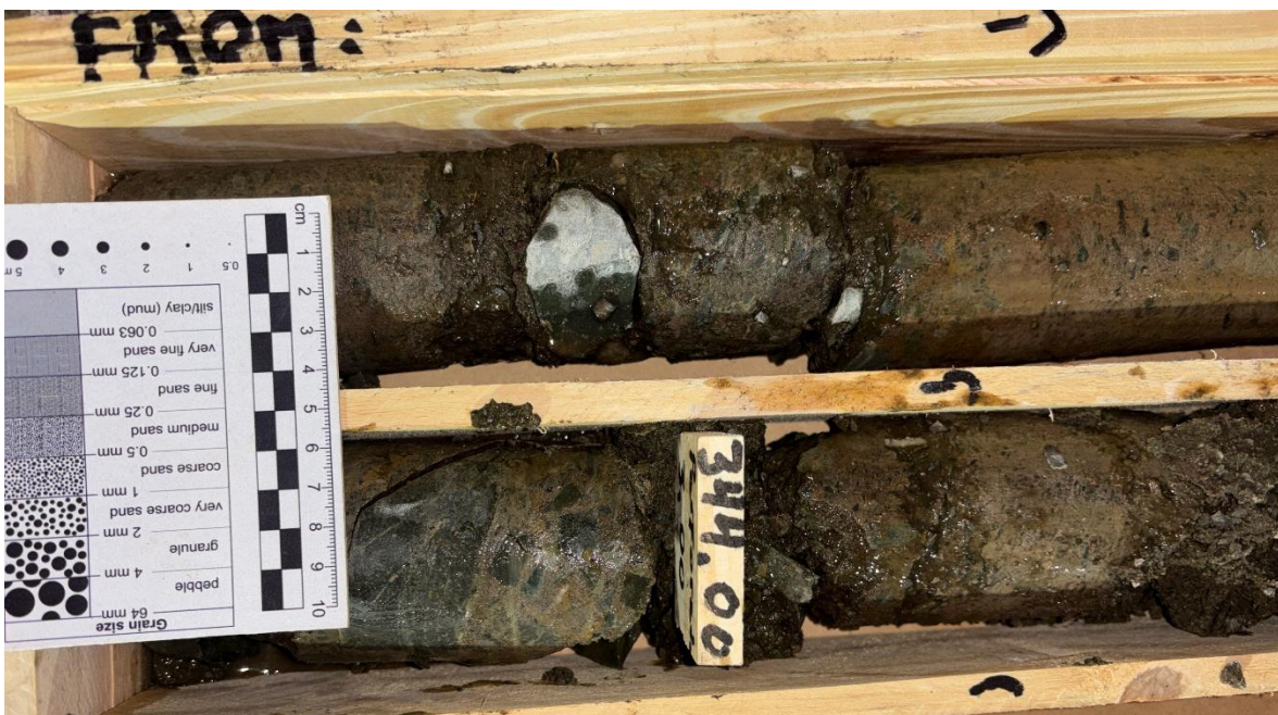
Figure 4. Angular pieces of gravel shows it was in a high energy environment when deposited
