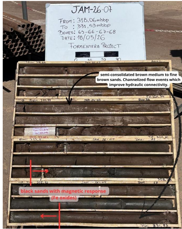
Figure 3. Sections show high porosity and connectivity
