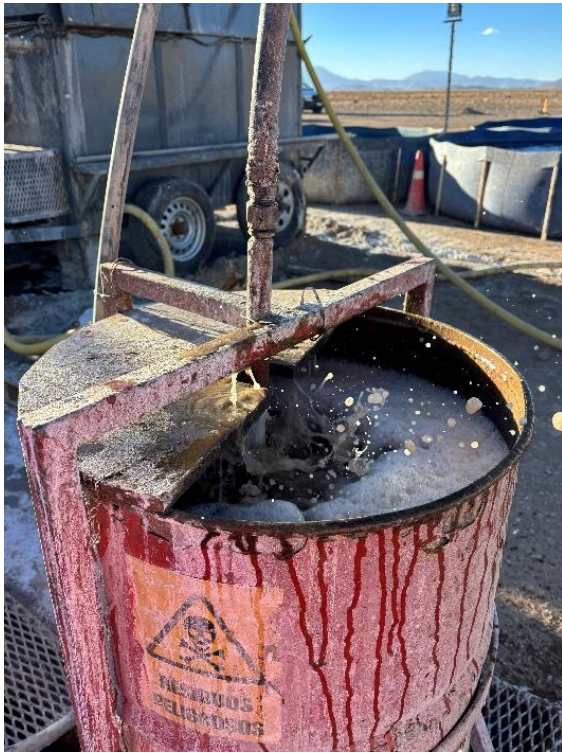
Figure 2. 11 th Packer test being conducted and brines flowing into one of the five tanks filled.
