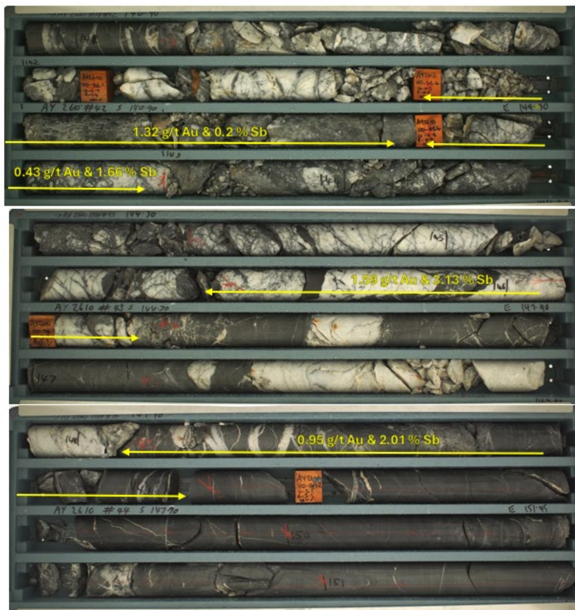
Figure 1: AY2610 significant intercepts annotated on core trays
