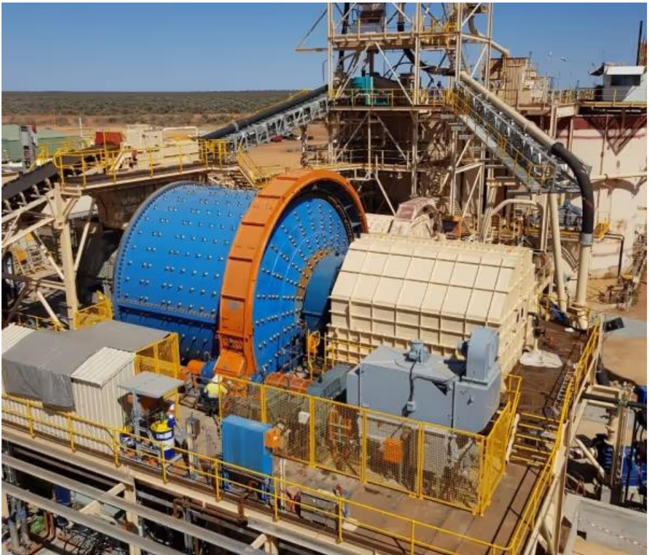
Figure 7. Kirkalocka SAG Mill (operated by Gylden Resources Pty Ltd)
