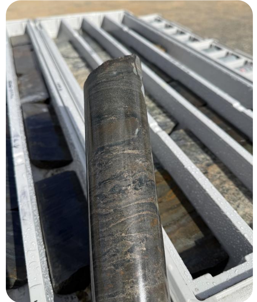
MTHD0003: Image from 180.5m with the interval assay returning 10.07 g/t Au
